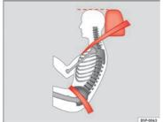
Fig. 14 Correct seat belt and head restraint positions, viewed from side
