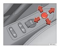
Fig. 90 Controls of exterior mirrors
