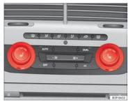
Fig. 96 Front seat heating with Climatronic
