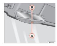
Fig. 89 Automatic antidazzle interior mirror.
