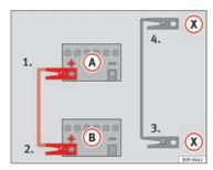
Fig. 203 Diagram for connecting jump leads if the vehicle providing assistance is fitted with the Start-Stop system: flat battery (a) and battery providing current (a).
