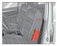
Fig. 22 Side airbag in driver seat
