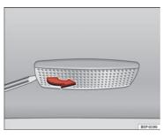
Fig. 200 Removing sun visor light
