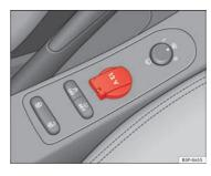
Fig. 118 Electric socket, centre console, front
