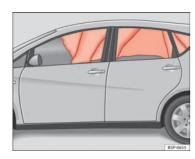
Fig. 25 Deployed curtain airbags
