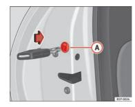
Fig. 60 Locking the doors manually
