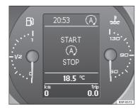
Fig. 139 Display on the instrument panel during Start-Stop function operation.
