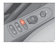
Fig. 149 Centre console: Switch for parking aid
