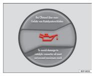
Fig. 164 In the engine compartment: Engine oil filler cap
