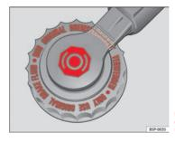
Fig. 171 In the engine compartment: Brake fluid reservoir cover
