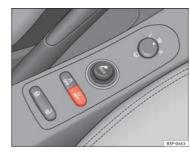
Fig. 52 Centre console: tyre monitor system but-
