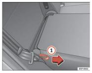
Fig. 99 Folding or opening the rear seat backr-
