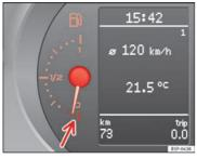
Fig. 35 Instrument panel: fuel gauge
