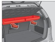
Fig. 124 Removing storage compartment
