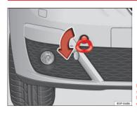
Fig. 204 The front right section of the vehicle: Fitting the front towing eye
