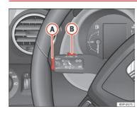
Fig. 150 Turn signal and main beam headlight lever: switch and rocker switch for the cruise con-
