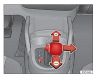
Fig. 146 Changing gear with tiptronic
