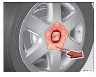
Fig. 175 Changing the wheel: Removing a hub cap
