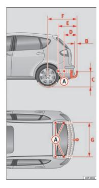
Fig. 156 Attachment points for towing bracket
