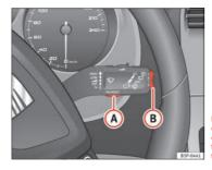
Fig. 47 Windscreen wiper lever (MFI): button A to confirm the menu selection and rocker switch B to change the menu
