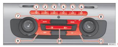
Fig. 132 On the dash panel: 2C Climatronic controls.
