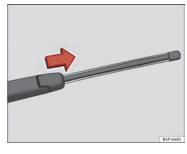
Fig. 169 Removing rear window wiper blade
