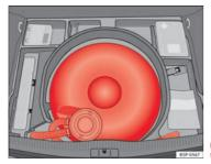
Fig. 159 LPG tank in spare wheel well
