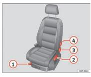
Fig. 94 Front left seat controls
