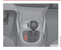
Fig. 142 Centre console: Selector lever for automatic gearbox / DSG automatic gearbox
