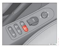
Fig. 137 Centre console: gas system control switch.
