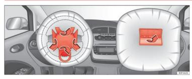
Fig. 21 Airbag covers reacting when the front airbags are triggered
