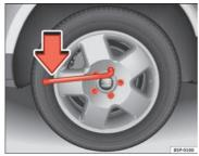
Fig. 176 Changing the wheel: loosen the wheel bolts
