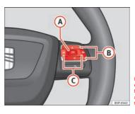
Fig. 46 Steering wheel controls: button A to confirm the menu selection and switch B to change the menu
