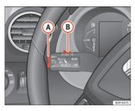
Fig. 151 Turn signal and main beam headlight lever: switch and rocker switch for the cruise control
