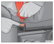
Fig. 16 Removing latch plate from buckle
