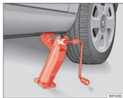
Fig. 178 Fitting the jack
