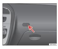
Fig. 27 Warning lamp for deactivated passenger airbag in centre console
