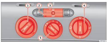
Fig. 125 Heating controls on the dash panel
