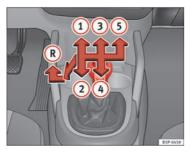
Fig. 140 Detailed view of the centre console: gear shift pattern of a 5-speed manual gearbox
