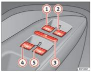
Fig. 69 Detail of the driver door: controls for the front and rear win-
