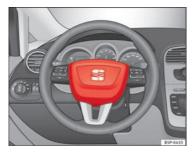
Fig. 18 Driver airbag located in steering wheel
