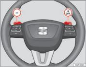
Fig. 147 Steering wheel with levers for automatic gearbox
