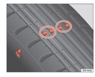
Fig. 172 Tyre tread wear indicators
