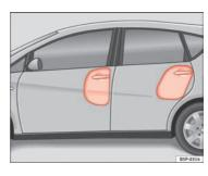
Fig. 23 Inflated side airbag on left side of vehicle
