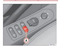
Fig. 138 The Start-Stop function button
