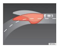
Fig. 76 Cornering lighting using adaptive headlights
