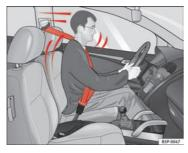
Fig. 11 A driver wearing the seat belt properly is secured by the belt in sharp braking
