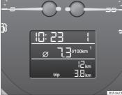
Fig. 42 Digital instrument panel display
