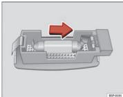
Fig. 201 Removing sun visor light
