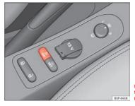
Fig. 135 Detailed view of the centre console: ESC (ESP) button
