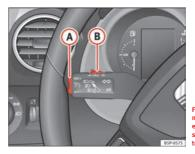
Fig. 154 Turn signal and main beam headlight lever: switch and rocker switch for the cruise con-
