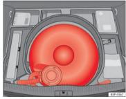
Fig. 158 LPG tank in spare wheel well
