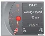
Fig. 35 Instrument panel: fuel gauge
