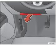
Fig. 179 Left side of dash panel: Fuse box cover
