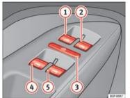
Fig. 69 Detail of the driver door: controls for the front and rear win-
