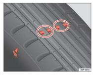
Fig. 171 Tyre tread wear indicators
