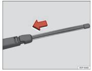
Fig. 169 Fitting the rear window wiper blade
