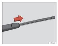
Fig. 168 Removing the rear window wiper blade
