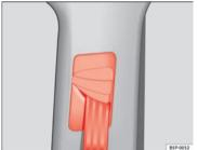
Fig. 17 Location of the belt height adjuster
