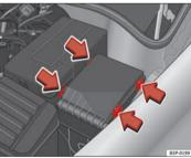
Fig. 180 Fuse box cover in engine compartment
