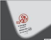
Fig. 6 Head restraint position warning label
