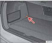
Fig. 32 Top Tether\* securing ring
