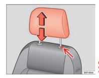
Fig. 92 Adjusting and removing the head restraints
