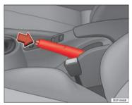
Fig. 147 Handbrake between the front seats
