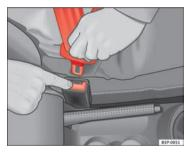
Fig. 16 Remove latch plate from buckle
