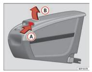
Fig. 113 Mobile storage compartment. Opening
