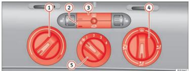
Fig. 124 Heating controls on the dash panel
