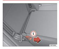
Fig. 99 Folding or opening the rear seat backrest
