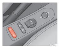
Fig. 59 Detailed view of the centre console: central lock button
