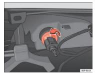
Fig. 193 Lamp on interior side of bumper
