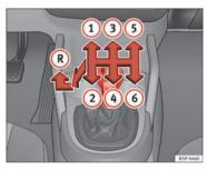
Fig. 140 Detailed view of the centre console: gear shift pattern of a 6-speed manual gearbox
