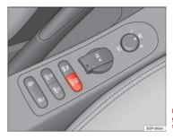
Fig. 136 Centre console: gas system control switch.
