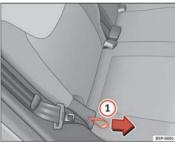
Fig. 97 Rear seat backrest angle adjustment
