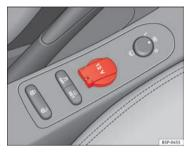
Fig. 117 Power socket, centre console, front
