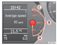
Fig. 36 Instrument panel: engine coolant temperature gauge
