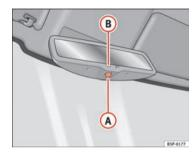
Fig. 88 Automatic antidazzle interior rear vision mirror.
