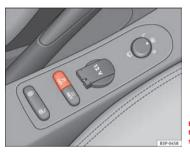
Fig. 134 Detailed view of the centre console: ESC switch.
