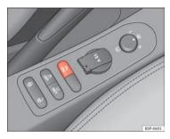
Fig. 148 Centre console: Switch for parking aid
