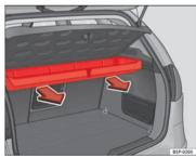
Fig. 123 Removing storage compartment
