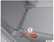
Fig. 98 Folding or opening the rear seat backr-
