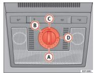
Fig. 70 Roof lining description: sliding/tilting sunroof rotary knob
