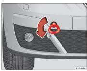
Fig. 203 The front right section of the vehicle: Fitting the front towline anchorage
