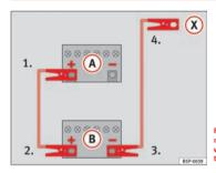
Fig. 201 Diagram of connections for vehicles without Start-Stop system
