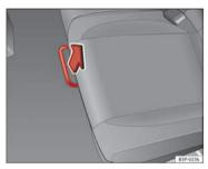
Fig. 96 For unlocking the rear seat
