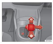
Fig. 145 Changing gear with tiptronic
