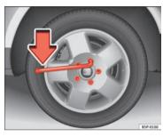
Fig. 175 Changing a wheel: loosen the wheel bolts
