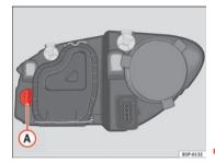
Fig. 182 Turn signal bulb
