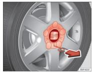
Fig. 174 Changing a wheel: Removing a hub
