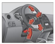
Fig. 132 Adjusting the steering wheel position
