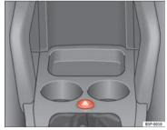
Fig. 76 Dash panel: switch for hazard warning
