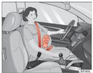
Fig. 15 Positioning seat belts during pregnancy
