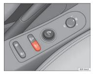
Fig. 52 Centre console: tyre monitor system button
