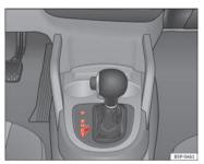
Fig. 141 Centre console: Selector lever for automatic gearbox / DSG automatic gearbox
