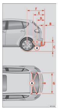
Fig. 155 Attachment points for towing bracket
