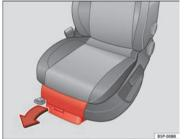
Fig. 102 Storage compartment under the front seats
