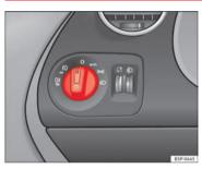
Fig. 72 Detailed view of the dash panel: lights, fog lights and rear fog light switch
