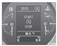
Fig. 138 Display on the instrument panel during Start-Stop function operation.
