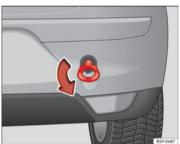
Fig. 204 Fitting the towline anchorage to the rear of the vehicle
