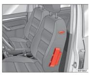
Fig. 22 Side airbag in driver seat
