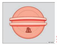
Fig. 164 In the engine compartment: Coolant expansion tank cap
