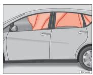
Fig. 25 Deployed curtain airbags
