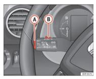
Fig. 149 Turn signal and main beam headlight lever: switch and rocker switch for the cruise control
