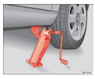
Fig. 177 Fitting the jack
