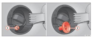
Fig. 157 Fuel tank open with LPG filler neck and adapter.
