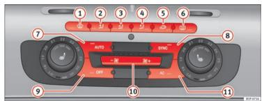
Fig. 131 On the dash panel: 2C Climatronic controls.
