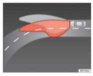
Fig. 75 Cornering lighting using adaptive headlights
