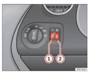
Fig. 74 Dash panel: regulation for instrument and switch lighting and headlight range control
