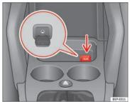
Fig. 118 Auxiliary audio connection
