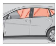
Fig. 25 Deployed curtain airbags
