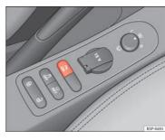
Fig. 153 Centre console: Switch for parking aid
