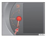
Fig. 35 Instrument panel: fuel gauge
