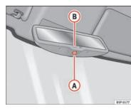
Fig. 87 Automatic antidazzle interior rear vision mirror
