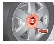
Fig. 179 Changing a wheel: Removing a hub
