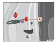
Fig. 58 Locking the doors manually
