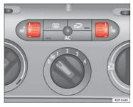
Fig. 93 Thumb wheel for the front seat heating
