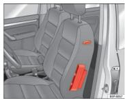
Fig. 22 Side airbag in driver seat
