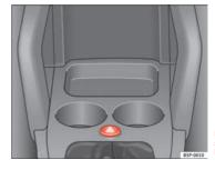
Fig. 74 Dash panel: switch for hazard warning lights
