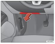
Fig. 185 Left side of dash panel: fuse box cover
