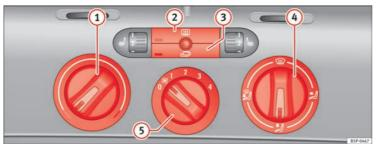
Fig. 129 Heating controls on the dash panel
