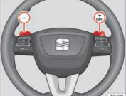
Fig. 151 Steering wheel with levers for automatic qearbox
