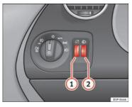
Fig. 72 Dash panel: regulation for instrument and switch lighting and headlight range control
