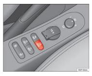
Fig. 141 Centre console: gas system control switch.
