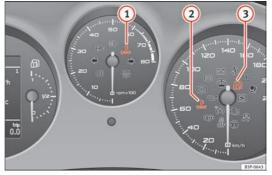
Fig. 49 Instrument panel control and warning lamps in vehicles with LPG
