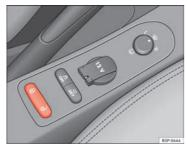
Fig. 57 Detailed view of the centre console: central lock button
