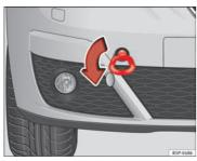
Fig. 216 The front right section of the vehicle: Fitting the front towline anchorage
