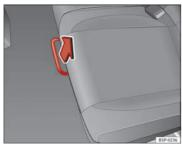
Fig. 95 For unlocking the rear seat
