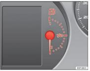
Fig. 37 Instrument panel: gas gauge.
