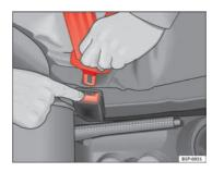
Fig. 16 Remove latch plate from buckle
