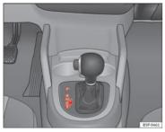
Fig. 146 Centre console: Selector lever for automatic gearbox / DSG automatic gearbox
