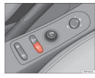
Fig. 50 Centre console: tyre monitor system but-
