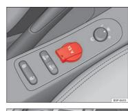
Fig. 117 Power socket, centre console, front
