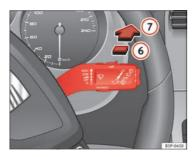
Fig. 86 Windscreen wiper and windscreen wash lever: rear window wiper
