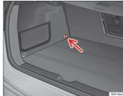
Fig. 32 Top Tether\* securing ring
