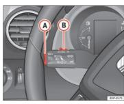
Fig. 154 Turn signal and main beam headlight lever: switch and rocker switch for the cruise con-
