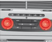
Fig. 94 Front seat heating with Climatronic
