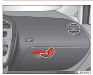
Fig. 100 Passenger side: storage compartment
