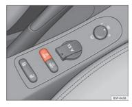
Fig. 139 Detailed view of the centre console: ESC switch.
