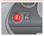
Fig. 70 Detailed view of the dash panel: lights, fog lights and rear fog light switch
