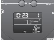
Fig. 44 Digital instrument panel display: average fuel consumption indicator
