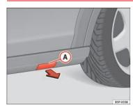
Fig. 183 Plastic sill panel trim with jack allotment cover
