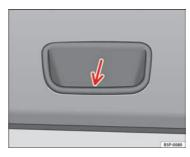
Fig. 65 Close-up of the inside trim of the rear lid: hand grip
