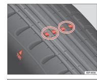
Fig. 176 Tyre tread wear indicators
