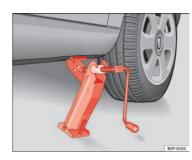
Fig. 182 Fitting the jack
