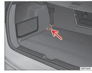
Fig. 128 Fastening rings for the separation net
