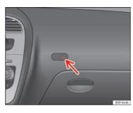
Fig. 27 Control lamp for deactivated front passenger airbag in centre console
