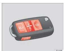
Fig. 47 Buttons on the key of vehicles with sliding doors.
