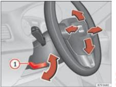
Fig. 133 Mechanical steering wheel adjustment.
