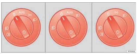
Fig. 67 Next to the steering wheel: diagram of some of the types of light switch.
