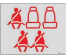
Fig. 4 Example of seat belt status display for the rear seats (here, a 7-seat vehicle) on the instrument panel. above the second row and below the third row of seats.
