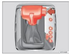
Fig. 140 Right-hand drive vehicles: Automatic gearbox selector lever with locking button (arrow).
