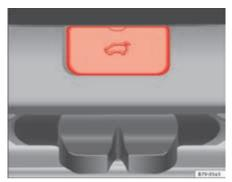
Fig. 200 From the luggage compartment: Remove the tailgate cover.
