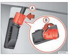
Fig. 224 Number plate light: To remove the lamp holder.
