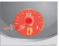
Fig. 169 On the instrument panel: Fuel gauge for petrol and diesel.
