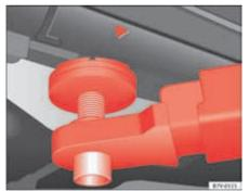
Fig. 168 Rear jacking points for raising vehicle with lifting platform or jack.
