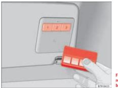
Fig. 64 Radio frequency remote control and control buttons on the sunshade.
