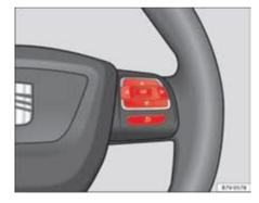
Fig. 39 Right side of multifunction steering wheel: Buttons to access the instrument panel menus.
