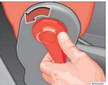
Fig. 89 Unlocking the folding backrest of the front passenger's seat.
