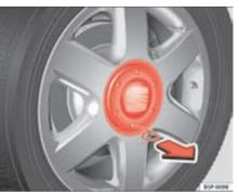
Fig. 186 Removing the hub cap.
