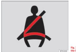
Fig. 3 Warning lamp on the instrument panel
