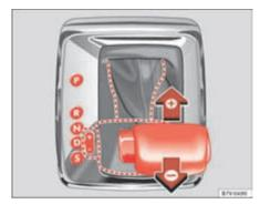
Fig. 141 Selector lever in Tiptronic position (lefthand drive vehicles). The lay-out in right-hand drive vehicles is symmetrically opposed.
