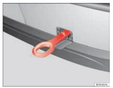
Fig. 229 On the rear bumper, to the right hand side: Tow ring in position.
