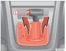
Fig. 204 Remove the lining from the area of the gear indication.
