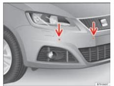
Fig. 149 Parking sensor system sensors on the front bumper.
