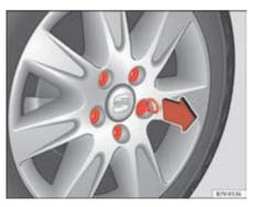
Fig. 189 Removing the wheel bolt caps
