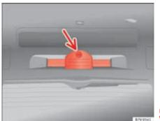
Fig. 196 On the boot lid: Warning triangle bracket.
