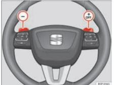
Fig. 142 Steering wheel with two paddle shifts for Tiptronic.
