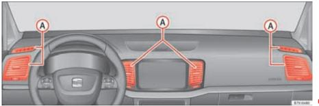
Fig. 131 Air vents in the instrument panel.
