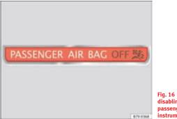
Fig. 16 Warning lamp for disabling the front passenger airbag on the instrument panel.
