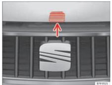
Fig. 174 Release lever to open the bonnet in the radiator grille.
