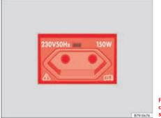
Fig. 127 Rear centre console: 230 Volt Euro socket.
