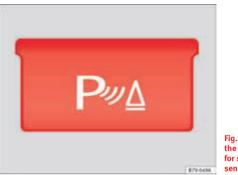
Fig. 148 Detailed view of the centre console: button for switching the parking sensor system on and off.
