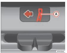
Fig. 201 From the luggage compartment: Manually unlocking the tailgate.
