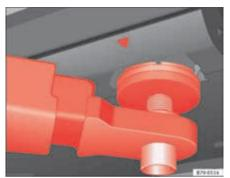
Fig. 167 Front jacking points for raising vehicle with lifting platform or jack.
