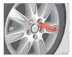
Fig. 194 Changing the wheel: loosen wheel bolts with the socket at the end of the wheel brace.
