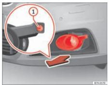
Fig. 217 On the righthand side of the front bumper: Removing the headlights
