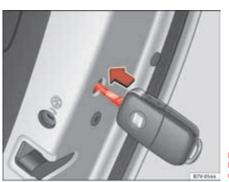
Fig. 199 Emergency locking of the vehicle using the vehicle key.
