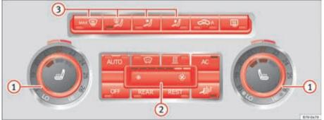
Fig. 130 Detailed view of the centre console: Climatronic controls.
