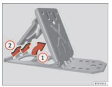
Fig. 208 To unfold the foldable wedges.
