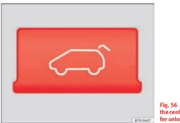
Fig. 56 Detailed view of the centre console: button for unlocking the tailgate.
