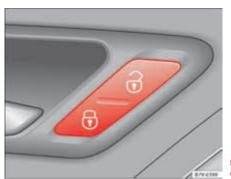
Fig. 48 In the driver door: central locking button.
