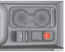
Fig. 125 Front centre console: lighter.
