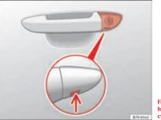
Fig. 197 Driver's door handle: Hidden lock cylinder.
