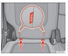
Fig. 28 Version 2: identification of the anchor points for the child seat on the vehicle seat.
