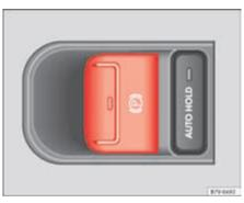
Fig. 143 Detailed view of the centre console: electronic parking brake switch
