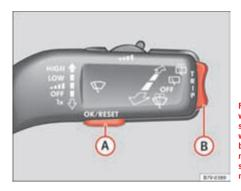
Fig. 38 In vehicles without multifunction steering wheel: On the windscreen washer lever: button (A) to confirm the menu point and rocker switch (B) to change the menu
