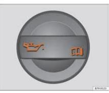
Fig. 176 In the engine compartment: Engine oil filler cap.
