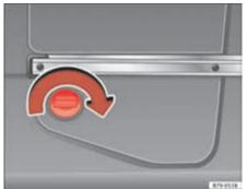
Fig. 171 At the rear left of the luggage compartment: AdBlue tank, behind a cover panel.
