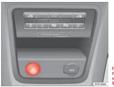
Fig. 135 Detailed view of the centre console: KESSY starter and lock system: Starter button.
