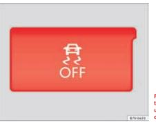
Fig. 144 Detailed view of the centre console: button used to switch TCS on and off (vehicles with ESP).
