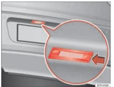
Fig. 223 On the rear bumper: number plate lights.
