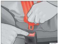
Fig. 11 Release the latch plate from the buckle.
