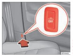
Fig. 51 Driver's seat: button for switching off the interior monitoring system and the anti-tow system.
