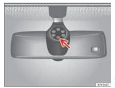
Fig. 76 Rain sensor sensitive surface.
