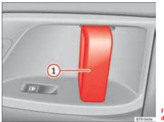
Fig. 53 On the sliding door. door handle 1.
