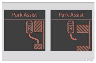
Fig. 153 Gap detected: Engage the reverse gear to park (parallel or nose/tail to the kerb).
