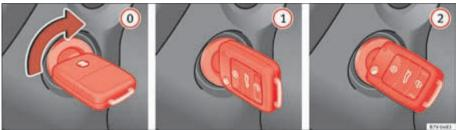
Fig. 134 Vehicle key positions
