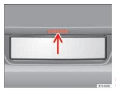
Fig. 57 Opening the tailgate from the exterior
