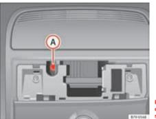
Fig. 203 Allen bolt to close the panoramic sliding roof.
