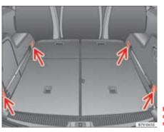
Fig. 101 In the luggage compartment: fastening rings
