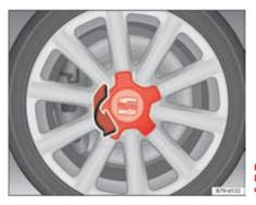
Fig. 187 Remove the hubcap by turning it outwards.
