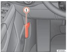
Fig. 173 In the footwell on the driver side: Lever for unlocking the bonnet.
