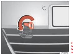
Fig. 228 On the righthand side of the front bumper: Screw in the towing ring.
