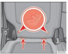
Fig. 27 Version 1: identification of the anchor points for the child seat on the vehicle seat.
