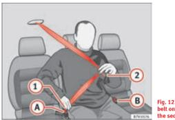
Fig. 12 Fasten the seat belt on the centre seat in the second row of seats.
