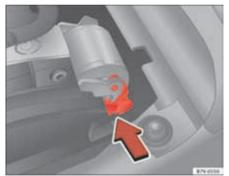
Fig. 205 Manual release of gear selector lever.
