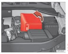
Fig. 181 In the engine compartment: Unfold the vehicle's battery hose.
