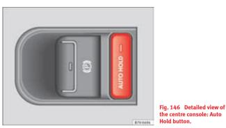
The control lamp on the button switches on when the Auto Hold function is on.
