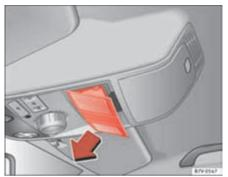
Fig. 202 On the interior roof lining: Remove cover.
