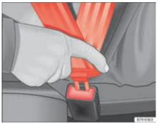
Fig. 10 Insert the latch plate into the buckle.
