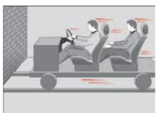
Fig. 5 Vehicle about to hit a wall: the occupants are not wearing seat belts.
