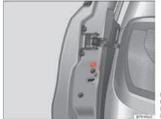
Fig. 198 To the front of the passenger side door: Emergency lock, hidden by a rubber cap.
