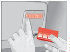
Fig. 65 To program: Press the buttons on the garage door control and the remote control simultaneously.
