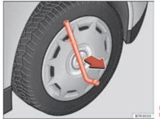
Fig. 188 Removing the full hubcap.
