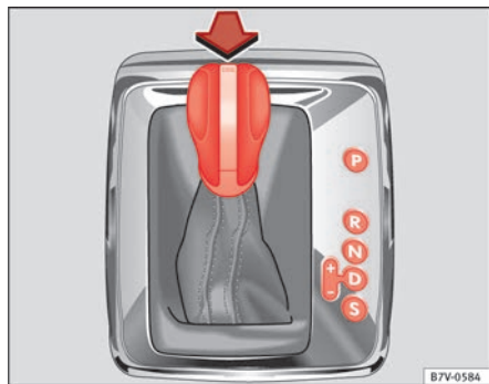
Fig. 132 Right-hand drive vehicles: Automatic gearbox selector lever with locking button (arrow).
