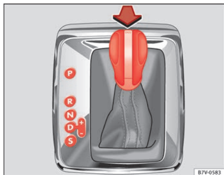
Fig. 131 Left-hand drive vehicles: Automatic gearbox selector lever with locking button (arrow).
