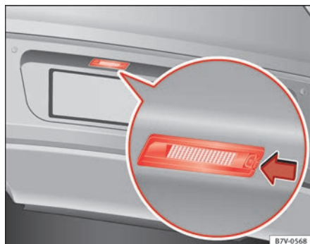
Fig. 213 On the rear bumper: number plate lights.
