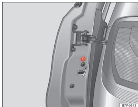
Fig. 189 To the front of the passenger side door: Emergency lock, hidden by a rubber cap.
