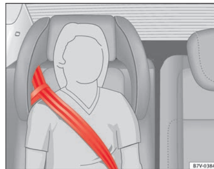
Fig. 32 Integrated child seats. seat belt routing with guide handle.
