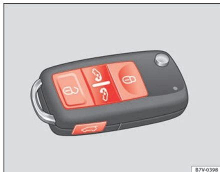
Fig. 46 Buttons on the key of vehicles with sliding doors.
