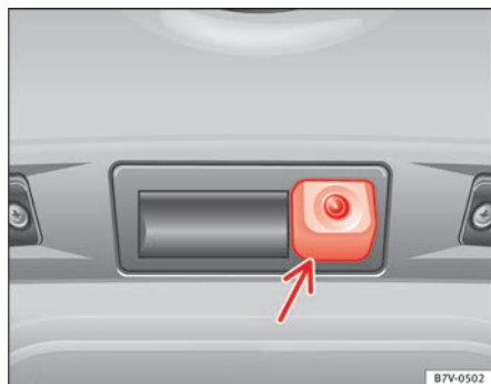
Fig. 146 On the boot lid: location of the rear assist camera.
