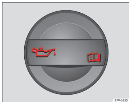
Fig. 169 In the engine compartment: Engine oil filler cap.
