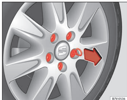
Fig. 180 Removing the wheel bolt caps
