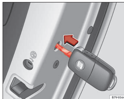
Fig. 190 Emergency locking of the vehicle using the vehicle key.
