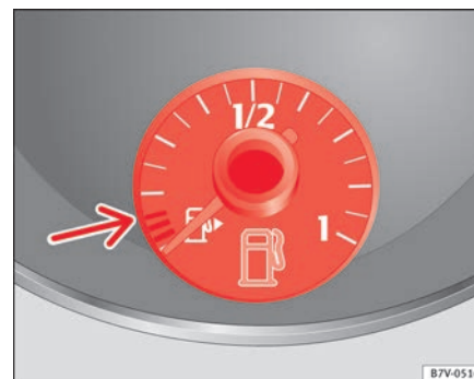
Fig. 162 On the instrument panel: Fuel gauge for petrol and diesel.
