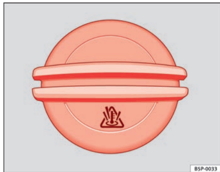
Fig. 172 In the engine compartment: Coolant expansion tank cap.
