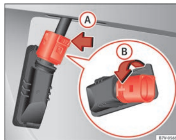
Fig. 216 Number plate light: To remove the lamp holder.
