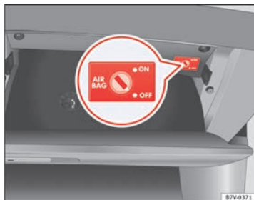
Fig. 19 In the glove compartment on the front passenger side: key switch for disabling and enabling the front passenger airbag.
