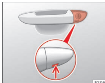
Fig. 190 Driver's door handle: Hidden lock cylinder.
