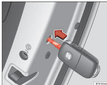
Fig. 192 Emergency locking of the vehicle using the vehicle key.
