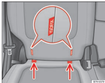
Fig. 27 Version 2: identification of the anchor points for the child seat on the vehicle seat.
