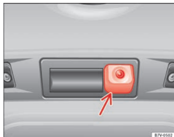
Fig. 147 On the boot lid: location of the rear assist camera.
