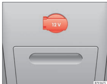
Fig. 120 Centre console, rear section: 12 volt power socket
