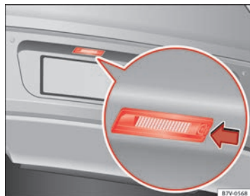
Fig. 215 On the rear bumper: number plate lights
