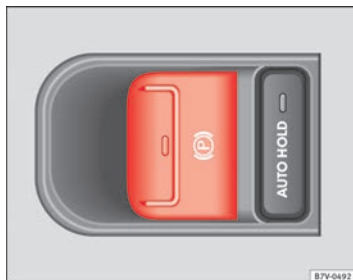
Fig. 136 Detailed view of the centre console: electronic parking brake switch
