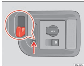
Fig. 99 In the luggage compartment: retaining hooks
