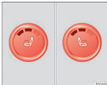
Fig. 78 Detailed view of the centre console: front seat heating controls, here with the second temperature level set
