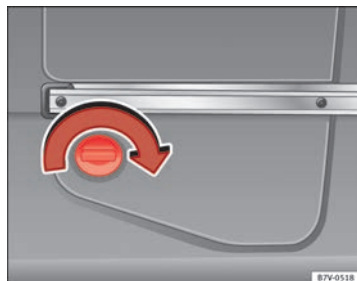
Fig. 166 At the rear left of the luggage compartment: AdBlue tank, behind a cover panel
