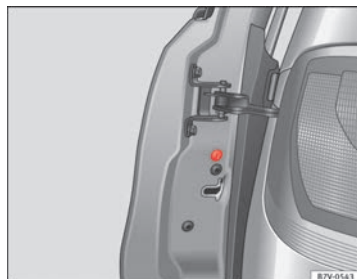
Fig. 191 To the front of the passenger side door: Emergency lock, hidden by a rubber cap
