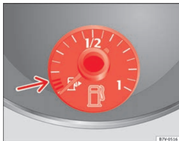
Fig. 164 On the instrument panel: Fuel gauge for petrol and diesel
