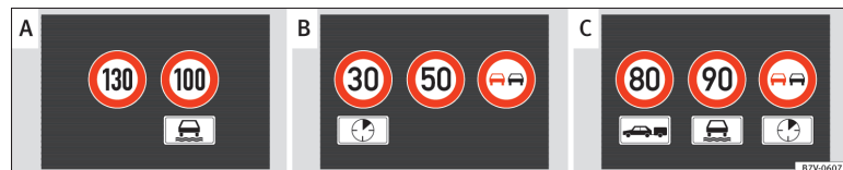
Fig. 154 Instrument panel display: Examples of speed limits or overtaking prohibitions detected together with the corresponding additional signs
