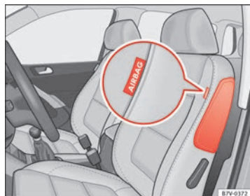
Fig. 20 On the side of the front seat: location of the side airbag
