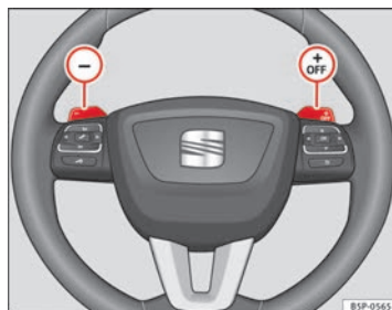
Fig. 135 Steering wheel with two paddle shifts for Tiptronic
