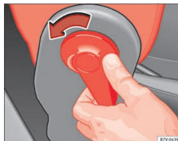
Fig. 83 Unlocking the folding seat backrest of the front passenger seat
