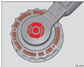
Fig. 138 In the engine compartment: brake fluid reservoir, lid
