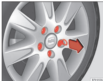
Fig. 182 Removing the wheel bolt caps
