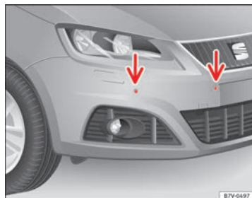
Fig. 142 Parking sensor system sensors on the front bumper
