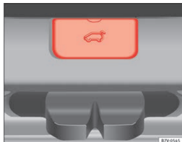
Fig. 193 From the luggage compartment: Remove the rear lid cover
