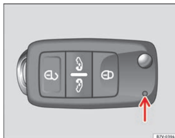
Fig. 42 Control lamp on the vehicle key for vehicles with electric sliding doors
