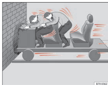
Fig. 6 The vehicle hits the wall: the vehicle occupants are not wearing seat belts
