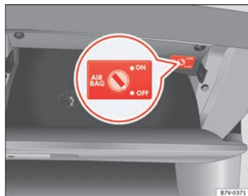
Fig. 19 In the glove compartment on the front passenger side: key switch for disabling and enabling the front passenger front airbag
