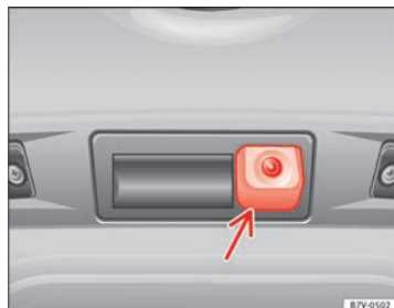
Fig. 147 On the rear lid: location of the rear assist camera
