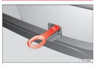
Fig. 104 On the rear bumper, to the right hand side: Towline anchorage in position
