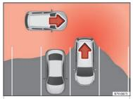
Fig. 224 Schematic representation of the rear cross traffic alert: monitored zone around the vehicle being parked.
