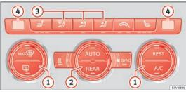
Fig. 52 Detailed view of the centre console: Climatronic controls
