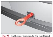
side: Towline anchorage in position
