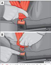
Fig. 87 Insert the latch plate into the buckle
