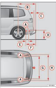
Fig. 231 Measurements and attachments to retrofit a tow hitch
