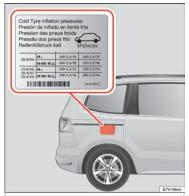
Fig. 251 Position of tyre pressure specification plate
