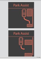
Fig. 213 Gap detected: engage the reverse gear to park (parallel or nose/tail to the kerb)
