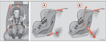
Fig. 36 On the rear seats: Possible installations for the child seat.
