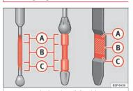
Fig. 241 Marked engine oil dipstick
