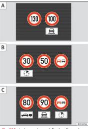
Fig. 225 Instrument panel display: Examples of speed limits or overtaking prohibitions detected together with the corresponding additional signs
