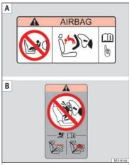
Fig. 35 Airbag stickers - version 2: on the front passenger's sun visor [A] and on the rear frame of the front passenger's door [B].
