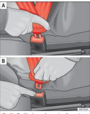
Fig. 21 Positioning and removing the seat belt buckle.
