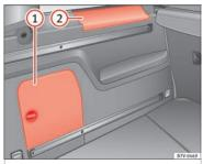
Fig. 187 In the luggage compartment: Side storage compartment
