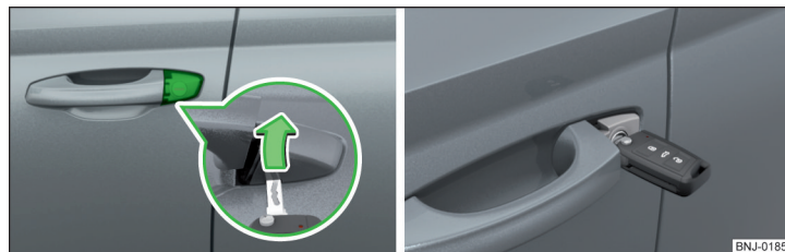
Fig. 193 Handle on the driver's door: opening lock cover / lock cylinder with key
