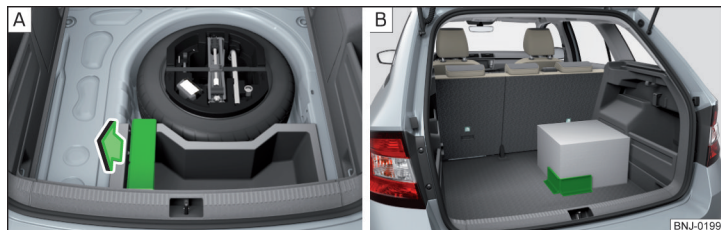
Fig. 100 Removing cargo element/example on how to mount the load by means of the cargo element
