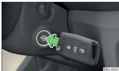
Fig. 115 Starting the engine - Press the button with the key
