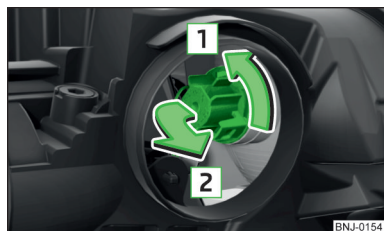
Fig. 209 Changing the bulb for the front turn signal light
