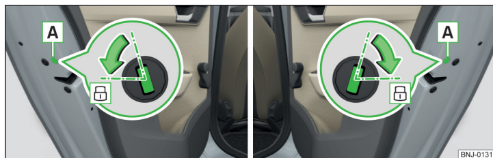
Fig. 194 Emergency locking: Left/right rear door
