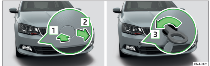
Fig. 190 Remove cap / install towing eye
