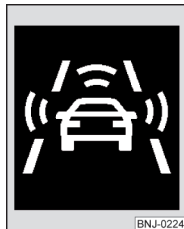
Fig. 146 Instrument cluster display: Warning or emergency braking at low speed
