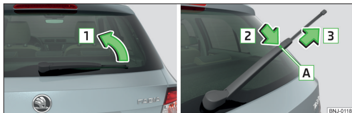
Fig. 199 Changing the rear window wiper blade
