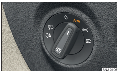
Fig. 42 Light switch: AUTO position
