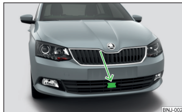
Fig. 125 Installation location of the radar sensor
