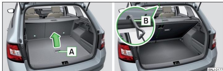
Fig. 104 Fold up variable loading floor / secure variable loading floor
