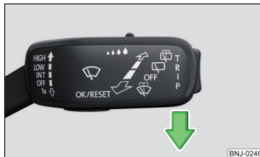
Fig. 197 Setting the service position for the wiper arms
