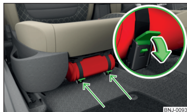
Fig. 179 Release the fire extinguisher
