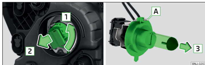
Fig. 213 Changing the bulb for the main beam
