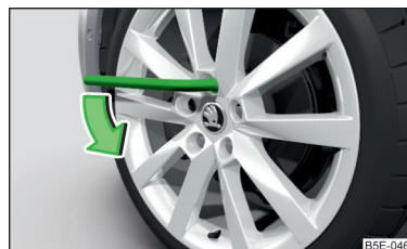
Fig. 184 Loosening the wheel bolts
