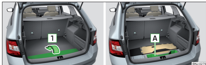
Fig. 99 Fold the floor back / storage compartment under the floor
