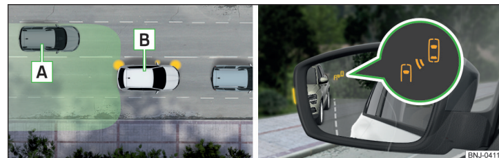
Fig. 212 Driving situation / indicator light in the left outside mirror indicates the driving situation
