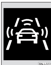
Fig. 228 Instrument cluster display: Warning or emergency braking at low speed
