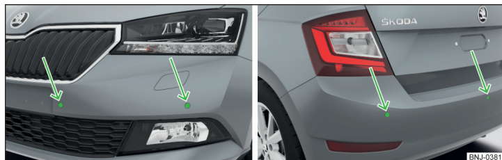
Fig. 205 Installation location of the sensors on the left side of the vehicle: front/rear
