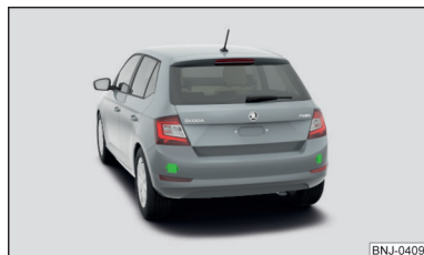
Fig. 210 Installation location of the radar sensors
