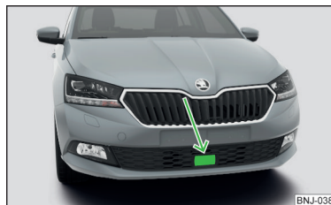
Fig. 203 Installation location of the radar sensor
