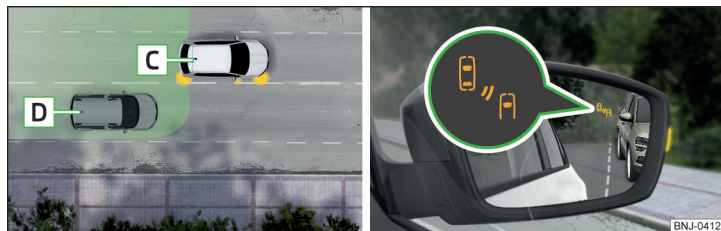
Fig. 213 Driving situation / indicator light in the right outside mirror indicates the driving situation
