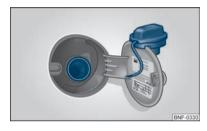
Fig. 89 Filler flap with tank cap unscrewed
