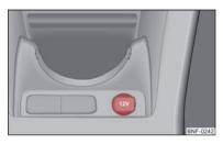
Fig. 44 Centre console: 12-Volt power socket
