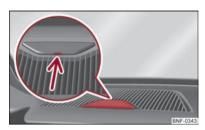
Fig. 69 Cap of the opening for the holder of the navigation unit
