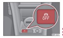
Fig. 66 Lower part of the centre console: Button for the City Safe Drive system
