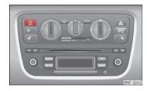
Fig. 64 Button for the START-STOP sys-
