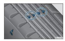
Fig. 99 Tyre tread with wear indicators
