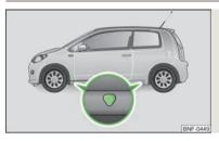
Fig. 112 Changing a wheel: Jacking points for positioning lifting jack
