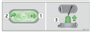
Fig. 123 Right side: Replacing the bulb for the turn signal light
