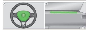
Fig. 83 Driver airbag in the steering wheel/front passenger airbag in the dashboard
