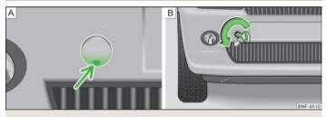
Fig. 118 Front bumper: Cap/installing the towing eye
