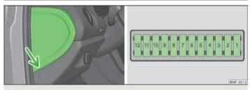
Fig. 121 On the driver's side of the dash panel: Fuse box cover/Schematic diagram of the fuse box
