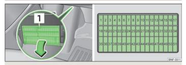
Fig. 119  $\,$  Underside of the dash panel: Fuse box/schematic diagram of the fuse box
