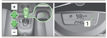
Fig. 75 Selector lever: manual shifting/instrument cluster: engaged gear
