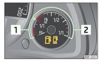
Fig. 5 Fuel gauge - CNG
