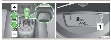
Fig. 72 Selector lever: manual shifting/instrument cluster: engaged gear
