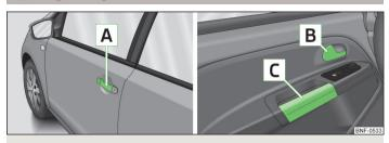
Fig. 11 Door handle/door opening lever:
