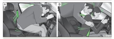
Fig. 87 Driver without a fastened seat belt/rear passenger without a fastened seat belt
