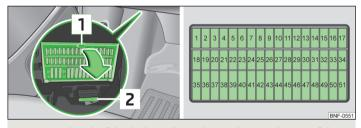
Fig. 124 Underside of the dash panel: Fuse box / schematic diagram of the fuse box
