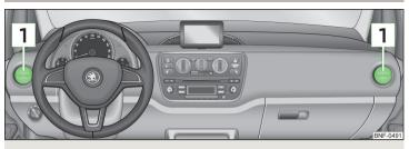
Fig. 71 Air outlet vents
