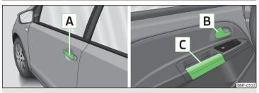
Fig. 28 Door handle/door opening lever:
