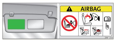
Fig. 12 Front passenger sun visor / label
