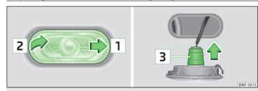
Fig. 128  $\,$  Left side of the vehicle: Replacing the bulb for the turn signal light
