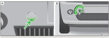
Fig. 115 Removing the cap/installing the towing eye
