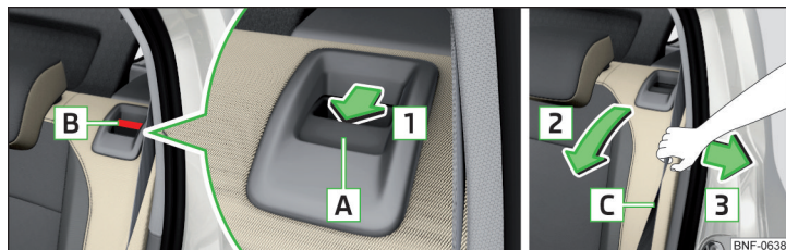
Fig. 50 Fold down seat backrest / pull on belt for side trim panel
