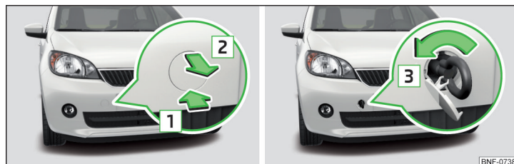
Fig. 127 Remove cap / install towing eye
