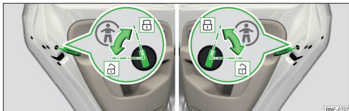
Fig. 30 Rear door: Child safety lock switch on / off
