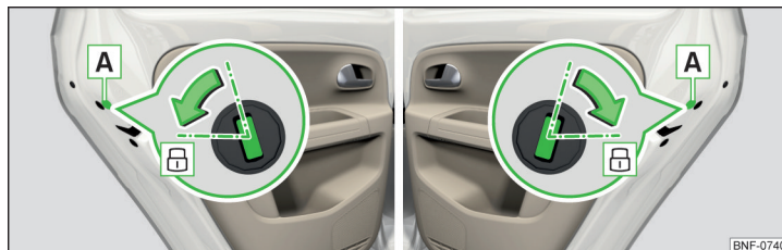
Fig. 129 Emergency locking: Left/right rear door
