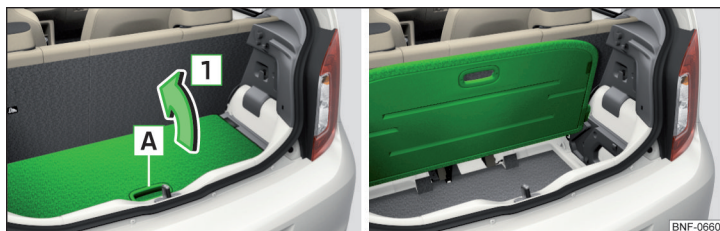
Fig. 77 Variable loading floor in the raised position: raise / raised
