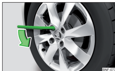
Fig. 121 Loosening the wheel bolts
