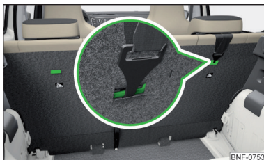
Fig. 14 Attachment points of the TOP TETHER system
