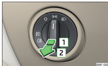
Fig. 39 Light switch - switch on front and rear fog light
