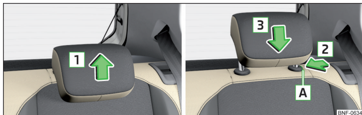
Fig. 51 Setting the height of the back headrest
