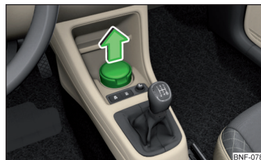
Fig. 63 Removing the ashtray
