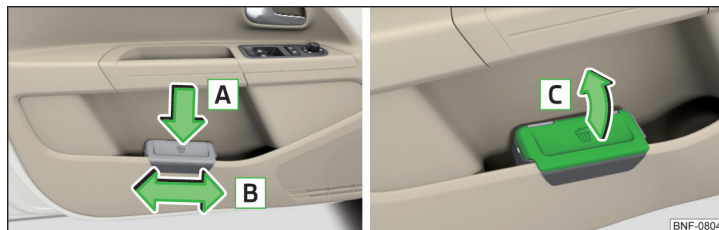
Fig. 60 Waste container: inserting and moving/opening
