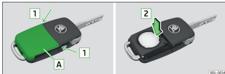
Fig. 128 Remove cover/take out battery
