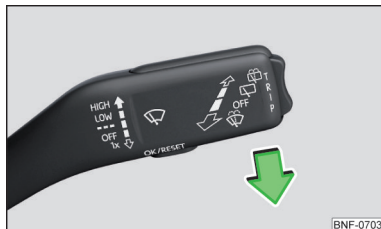
Fig. 131 Setting the service position for the wiper arms
