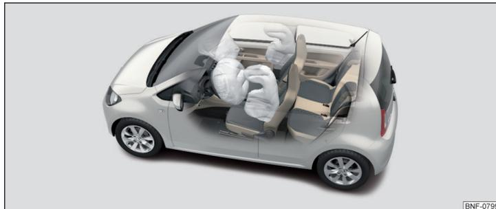
Fig. 7 Airbags rellenos de gas
