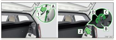
Fig. 81 Remove the luggage compartment cover
