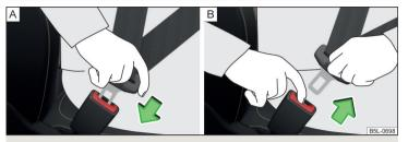
Fig. 5 Fastening/unfastening the seat belt
