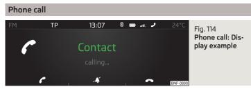
The device makes it possible to take another incoming call during an ongoing call. The existing telephone call is put on hold. You can switch between calls.
