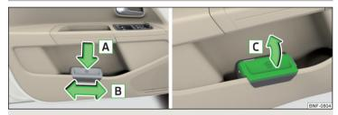
Fig. 62 Waste container: inserting and moving/opening
