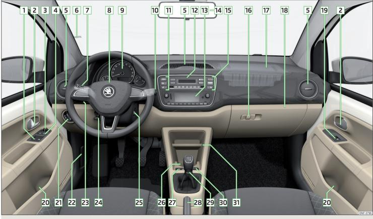
Fig. 15 Cockpit example for LHD models
