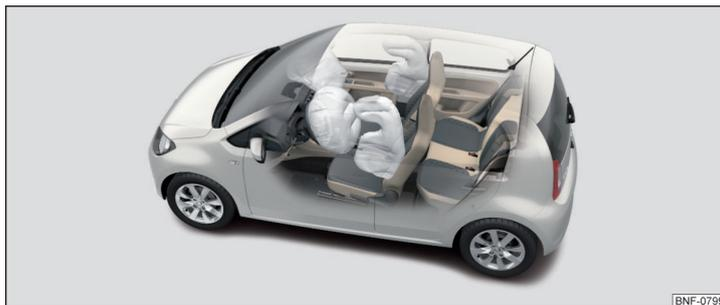
Fig. 9 Airbags rellenos de gas
