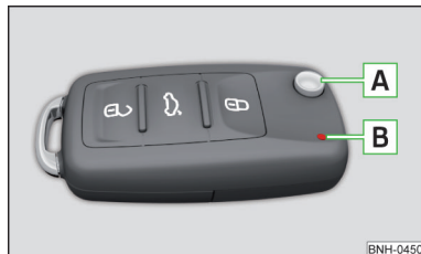
Fig. 29 Key with pop-out key bit
