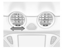
Adjust the air amount at the vent outlet by turning the adjuster wheel. The vent is closed when the adjuster wheel is turned close to the left or right.
