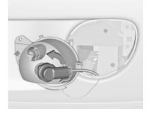
3. Disengage and remove the bulb socket by turning anticlockwise.
