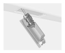
Remove lamp downwards, taking care not to pull on the cable.
