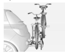
The rear carrier system (Flex-Fix system) allows one bicycle to be attached to a pull-out carrier integrated into the vehicle floor. It is possible to attach one further bicycle on an adapter. The transportation of other objects is not permitted.
