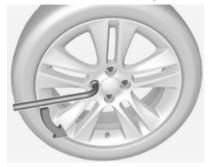
Install the wheel wrench ensuring that it locates securely and loosen each wheel bolt by half a turn.
