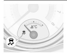
ESC is operational after each engine start as soon as the control indicator \$\mathcal{z}\$ extinguishes.
