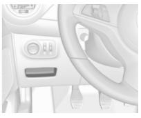
Storage compartments are located below the light switch, in the centre console in front of the gear selector lever, in the door pockets and in the side panels near the rear seats.
