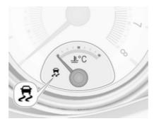
TC is operational after each engine start as soon as the control indicator \$\mathcal{z}\$ extinguishes.
