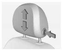
Press release button, adjust height, engage.
