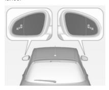
Side blind spot alert is active from speeds of 10 km/h up to 140 km/h. Driving faster than 140 km/h deactives the system, indicated by low lighting warning symbols at in both exterior mirrors. Reducing the
