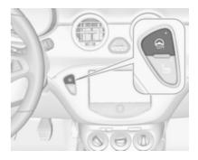
Press button ⊕ when engine is running. The system works from standstill up to 35 km/h, and in reverse gear. Above this speed the system changes to normal mode. When activated, City mode engages automatically below 35 km/h.
