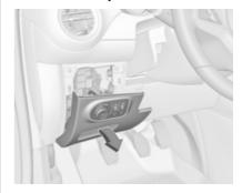
In left-hand drive vehicles, the fuse box is behind the light switch in the instrument panel.
