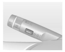
Press the **MENU** button to switch between the menus or to return from a submenu to the next higher menu level.
