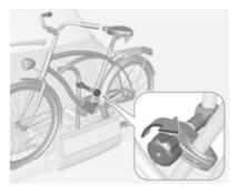
Attach the short mounting bracket to the bicycle frame. Turn the knob clockwise to fasten.
