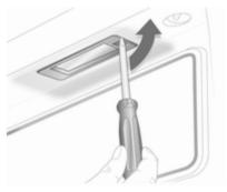
Insert screwdriver in recess of the cover, press to the side and release spring.
