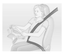
The seat belts are locked during heavy acceleration or deceleration of the vehicle holding the occupants in the sitting position. Therefore the risk of injury is considerably reduced.
