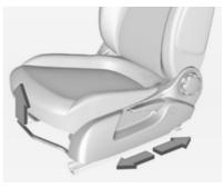
Pull handle, slide seat, release handle. Allow seat to engage in position.
