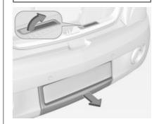
Pull release lever up. The system disengages and travels quickly out of the bumper.
