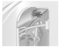
2. Unscrew the plastic securing nut from the inside by hand.
