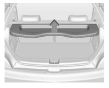
Lift up the cover at the rear end. It engages in a nearly vertical position. Further opening up to head restraints is possible. To close, move down the cover beyond the engage point.
