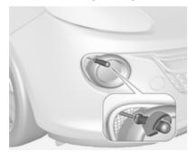
1. Undo screw and remove cover.
