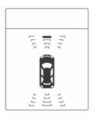
In the Driver Information Centre, the distance to a front and rear obstacle is displayed by changing distance lines.
