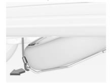
6. Lift the spare wheel holder a bit by hand and detach the safety cable.
