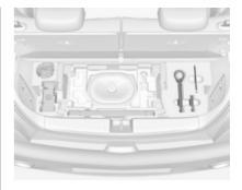
On version with subwoofer box, the tools and the towing eye are located together with the tyre repair kit and the warning triangle in the box below the floor cover. To gain access, remove floor cover: fold rear part to the front and pull out the cover to the rear \$\infty\$ 65.
