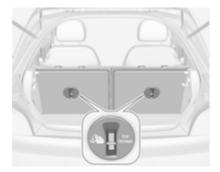
In addition to the ISOFIX mounting, fasten the Top-Tether strap to the Top-Tether fastening eyes.
