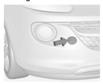
Disengage the cap by pushing on the marked position.
