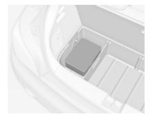
On versions with storage box in the load compartment the suitcase with the tyre repair kit is located in a chamber of the box  $\diamondsuit$  63.
