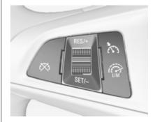
Press button @. If cruise control has been activated before, it is switched off when speed limiter is activated and the control indicator (©) extinguishes.
