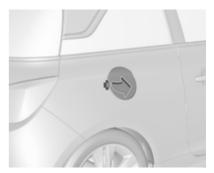
The fuel filler flap can only be opened when the vehicle is unlocked.
