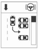
A brief vibration in the steering wheel after engaging reverse gear indicates that the steering is controlled by the system. Then the vehicle is steered into the slot automatically by giving the driver detailed instructions for braking, accelerating and gear shifting. The driver must keep hands away from the steering wheel.
