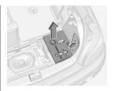
To gain access to the right cover in the load compartment, e.g. for bulb replacement, fold down rear right backrest and pull out the tool box beside the subwoofer.
