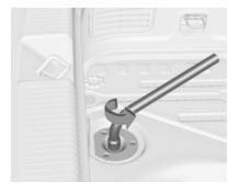
Fit the wheel wrench on the hexagon bolt near the tool box and turn it anti-clockwise until a resistance is noticeable.
