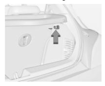
Use the hook at the right sidewall of the load compartment for hanging up carrier bags. Maximum load: 5 kg
