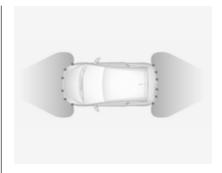
The system has six ultrasonic parking sensors each in the rear and front bumper.
