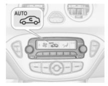
Climate control settings are shown on the Graphic-Info-Display, or depending on the version, on Colour-Info-Display. Setting modifications are briefly popped-up in both displays, superimposed over the currently displayed menu.
