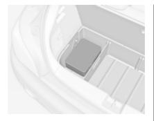
On version with storage box, the suitcase with the tools, the towing eye and the tyre repair kit is located in a chamber of the box in the load compartment ▷ 63.
