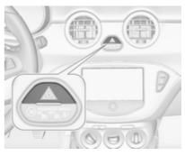
Operated by pushing the <u>A</u> button. In the event of an accident with airbag deployment the hazard warning flashers are activated automatically.
