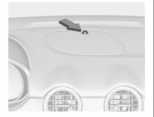
Status LED is integrated in the sensor on top of the instrument panel.
