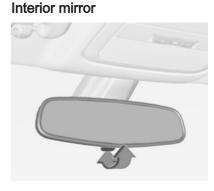
To reduce dazzle, adjust the lever on the underside of the mirror housing. Interior mirror \$\Display 27\$, Automatic antidazzle interior mirror \$\Display 28\$.
