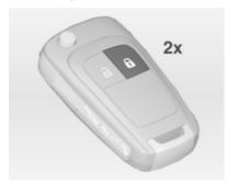
Press button non the radio remote control twice within 15 seconds.
