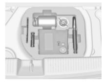
Some tools and the towing eye are located together with the tyre repair kit in a tool box in the load compartment below the floor cover. On version with storage box, remove box first ⇔ 63.
