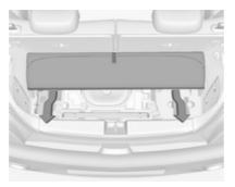
Remove floor cover to gain access to the tool box ▷ 170, tyre repair kit ▷ 177 and for bulb replacement of tail lights:
