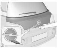
Press the brand emblem at the bottom half to unlock and open the tailgate.
