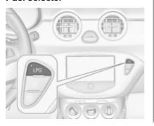
Pressing the **LPG** button switches between petrol and liquid gas operation as soon as the required parameters (coolant temperature, gas temperature and minimum engine speed) have been reached. The requirements are usually fulfilled after approx. 60 seconds (depending on exterior temperature) and the first firm press on the accelerator. The LED status shows the current operating mode.
