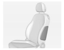
The side airbag system consists of an airbag in each front seat backrest. The location is identified by the word **AIRBAG**.
