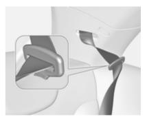
Insert seat belt latch plate into side holder to protect the belt against damage.
