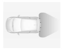
The system has four ultrasonic parking sensors in the rear bumper.
