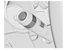
Press the **SET/CLR** button, the **MENU** button or turn the adjuster wheel to confirm a message.
