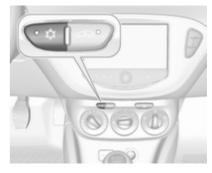
Press button to switch on cooling. Activation is indicated by the LED in the button. Cooling is only functional when the engine is running and climate control fan is switched on.
