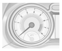
Displays the engine speed.
