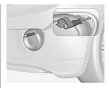
1. Undo screw and remove cover.
