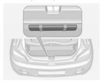
The warning triangle is stowed with elastic straps in the load compartment below the tailgate.
