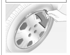
Alloy wheels: Disengage wheel bolt caps with a screwdriver and remove. To protect the wheel, place a soft cloth between the screwdriver and the alloy wheel.
