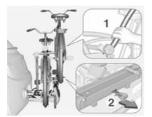
Hold frame (1) of rear bicycle with one hand and pull the loop (2) to disengage.
