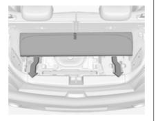
On versions with subwoofer box the tyre repair kit is located in the box under the floor cover in the load compartment. To use tyre repair kit, firstly remove floor cover: fold rear part to the front and pull out the cover to the rear  $\diamondsuit$  65.
