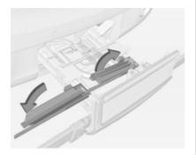
Remove strap and fold out the wheel recess.
