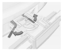
Remove strap and swivel both clamping levers sidewards as far as it will go.
