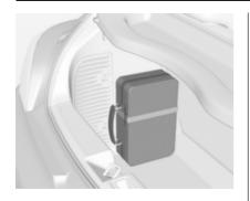
On versions with rear carrier system or liquid gas engine, the tools are located together with the towing eye and tyre repair kit in a suitcase, fixed with a strap at the left sidewall in the load compartment.
