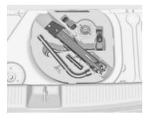
The jack, the wheel bolt wrench, the tools and two straps for securing a damaged wheel are in the tool box below the load compartment floor cover ♀ 65.
