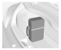
On versions with rear carrier system or liquid gas engine, tyre repair kit is located in a suitcase and fixed with a strap at the left sidewall in the load compartment.
