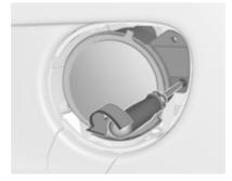
2. Undo screw and remove light assembly from the bumper.
