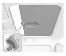
Press the button in the handle to open the sunblind and guide it backwards. It rolls up automatically.
