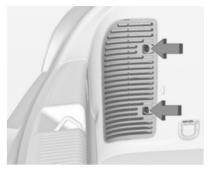
1. Release the cover on the respective side and remove.
