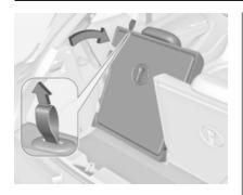
Pull the strap on one or both backrests and fold them down onto the seat cushion.
