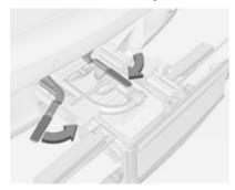
Swivel both clamping levers inwards as far as it will go. Fasten strap.
