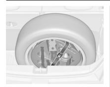
Position the tool box in the inside of the wheel and secure it with strap 2 inserted through two spokes of the wheel.
