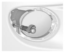
2. Undo screw and remove light assembly from the bumper.
