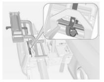
Guide the strap attached to the adapter underneath the lever for folding back the rear carrier system. Fasten the strap.
