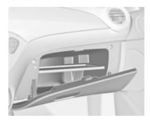
Pull lever to open the glovebox cover.
