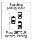
When searching for a parking slot, select parallel or perpendicular parking slot by pressing **SET/CLR** button on the turn signal lever.
