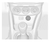
A 12 Volt power outlet is located in the centre console.
