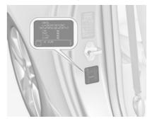
The identification plate is located on the left door frame.
