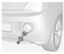
Insert a screwdriver in the slot at the lower bend of the cap. Disengage the cap by carefully moving the screwdriver downwards.
