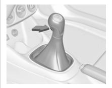
To engage reverse, with the vehicle stationary wait 3 seconds after depressing the clutch pedal and then press the release button on the selector lever and engage the gear.
