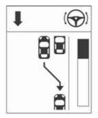
When a slot is detected, a visual feedback in the Driver Information Centre or Colour-Info-Display and an acoustic signal is given.
