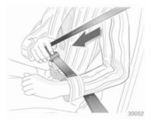
Withdraw the belt from the retractor, guide it untwisted across the body and insert the latch plate into the buckle. Tighten the lap belt regularly while driving by pulling the shoulder belt
