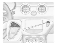
Press button **LPG** to switch between petrol and liquid gas operation. The LED in the button shows the current operating mode.
