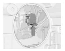
Press the clip to disengage bulb holder. Withdraw the bulb holder from the reflector.
