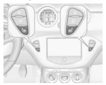
Activate seat heating by pressing ## button for the respective front seat.
