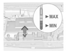
Different dipsticks are used depending on engine variant. When the engine oil level has dropped to the **MIN** mark, top up engine oil.
