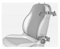
Turn handwheel to adjust inclination. Do not lean on backrest while adjusting.
