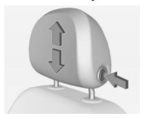
Press release button, adjust height, engage.
