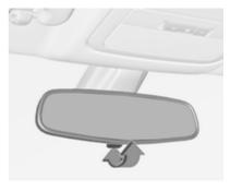
To reduce dazzle, adjust the lever on the underside of the mirror housing to the front or rear. Lever in the middle position is the normal driving position.
