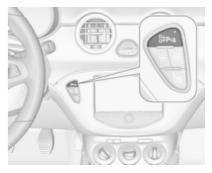
Front-rear parking assist and advanced parking assist both use the same button for activation and deactivation:
