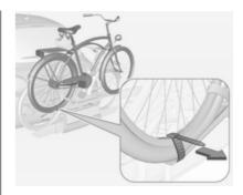
Additionally secure both bicycle wheels of the rear bicycle to the wheel recesses using the tensioning straps.
