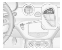
When searching for a parking slot, the system is ready to operate with a long press of button \$\text{BP}\_4\$.
