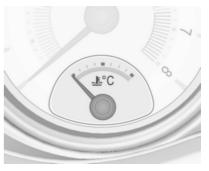
Displays the coolant temperature.
