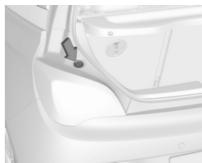
Fit light assembly with the retaining pins into the recesses of the vehicle body and tighten the securing nut from inside the load compartment. Pull the circular gasket over the recess in the lamp housing.
