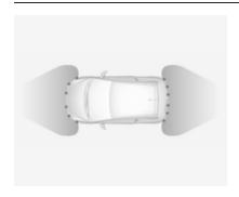
Advanced parking assist is always combined with front-rear parking assist, see previous section. Both systems use the same sensors in the front and rear bumper.
