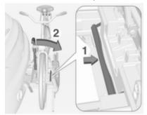
Push the lever (1) to disengage and hold.
