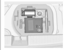
The tyre repair kit is in the tool box under the floor cover in the load compartment.
