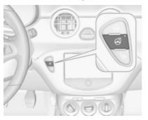
Activate heating by pressing button. Activation is indicated by the LED in the button.
