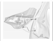
Carefully withdraw the light assembly from the recesses and remove.
