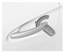
Manually unlock the driver's door by turning the key in the lock. Switch on the ignition and press the central locking button to unlock the passenger door, load compartment and fuel filler flap. By switching on the ignition, the anti-theft locking system is deactivated.
