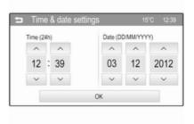
To adjust the time and date settings, tap on the  $\wedge$  and  $\vee$  screen buttons.
