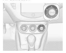
Turn right rotary knob for desired adjustment. Setting is indicated in the Info-Display.
