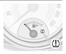
A detected low tyre pressure condition is indicated by the control indicator 1  $\Rightarrow$  86.
