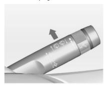
= automatic wiping with rain sensor
