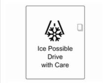
If outside temperature drops to 3 °C, a warning message is displayed in the Driver Information Centre with Uplevel-Display.
