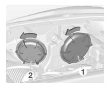
Low beam outer bulb (1). High beam inner bulb (2).
