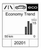
■ Economy Trend: Displays the average consumption development over a distance of 50 km. Filled segments display the consumption in 5 km steps and shows the effect of topography or driving behaviour on fuel consumption.
