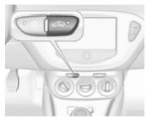
Press button to activate air recirculation mode. Activation is indicated by the LED in the button.
