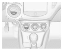
Press button \$\simetex\$ to activate air recirculation mode. Activation is indicated by the LED in the button.
