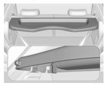
Push cover upwards at the left and right from the lower side and remove.
