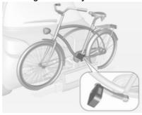
Rotate the pedals into position as shown in the illustration and put the bicycle on the wheel recess.
