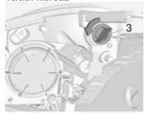
Rotate bulb socket (3) anticlockwise to disengage. Withdraw the bulb socket from the headlamp housing.
