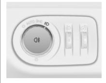
Operated by pushing the <code>Q‡</code> button. Light switch in position **AUTO**: switching on rear fog light will switch on headlights automatically.
