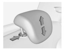
Pull the head restraint upwards and let engage. To move downwards, press the catch to release and push the head restraint downwards.
