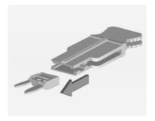
Place the fuse extractor on the various types of fuse from the top, and withdraw fuse.
