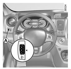
On vehicles fitted with this function, control **A** allows you to adjust the height of the beams according to the load.
