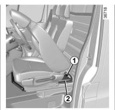
The tools included in the tool kit depend on the vehicle. The tool kit 2 is located under the driver's seat. To remove it. move the seat forward and fold down the seatback (refer to the information on the "Front seats" in Section 1). Unscrew the mounting screw 1 from the unit and swivel to extract.
