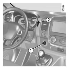
The RENAULT card must be inserted in card reader 2 or in detection zone 3.
