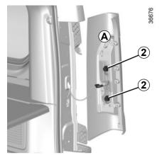
Turn the light unit slightly and release it to access the bulb holder **2**.
