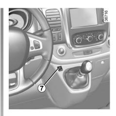
Vehicles fitted with the ECO mode (button 7): Once activated, ECO mode may reduce the effective performance of the heating and/ or air conditioning. Please refer to the information on "Driving advice, Eco-driving" in Section 2.
