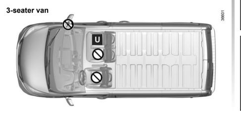
Check the status of the air bag before fitting a child seat or allowing a passenger to use the seat.
