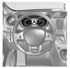
Instrument panel A: lights up when the ignition is switched on. The brightness can be adjusted by turning control knob 1.
