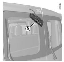
Remove the light sideways from the outside to access bulb **9**.
