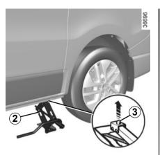
Insert the jack 2 horizontally; the jack head pin 3 should line up with the hole in the lower part of the bodywork nearest the wheel concerned.
