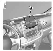
If necessary, lower the base **9** of the holder **8** to extend it.
