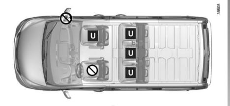
RISK OF DEATH OR **SERIOUS INJURY:** before fitting a rear-facing child seat on the front passenger seat, check that the airbag has been deactivated (please refer to the information on "Child safety: front passenger airbag deactivation, activation" in Section 1).
