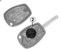
Replace battery **2** according to the direction marked on the cover.
