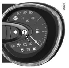
When fitted to the vehicle, this system notifies the driver if one or more tyres lose pressure.
