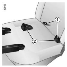
The two rings 1 are located between the seatback and the seat base of the seat and are identified by a marking .
