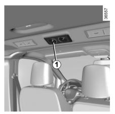
On equipped vehicles, there are four adjustable air vents and controls **1**.
