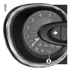
An overall rating from 0 to 100 is displayed to let you assess your eco driving performance. The higher the rating, the lower the fuel consumption.
