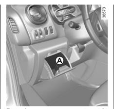
**Fuses in passenger compartment A** If any electrical component does not work, check the condition of the fuses. Unclip the storage **A**.
