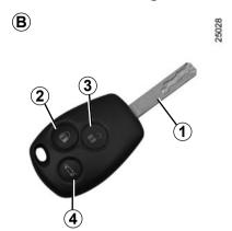
4 Locks/unlocks the boot and, depending on the vehicle, the side sliding door.
