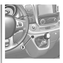
Vehicles fitted with the ECO mode (button 9): Once activated, the ECO mode may reduce the effective performance of the air conditioning. Please refer to the information on "Driving advice, Eco-driving" in Section 2.
