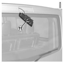
Remove the light from the outside to access the bulb **11**.
