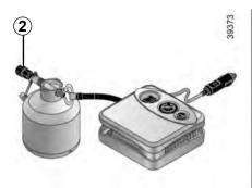
If a minimum pressure of 1.8 bar is not reached after 15 minutes, repair is not possible; do not drive the vehicle but contact an approved dealer.
