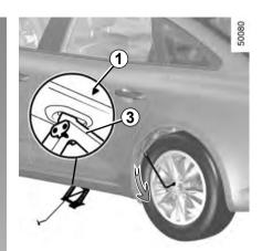
Crank up the jack by hand at first to align the base plate (which should be inclined further inwards than the jack head).
