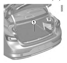
In the event of a puncture, use the kit located under the trunk carpet 1.
