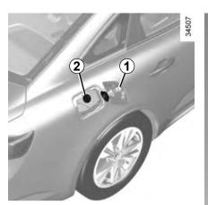
With the vehicle unlocked, to open cover 1, press area A then release. The cover 1 opens.
