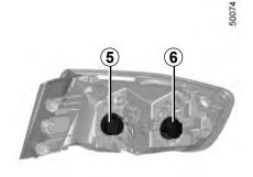
Refit the bulb holder and push the light unit in as far as it will go.
