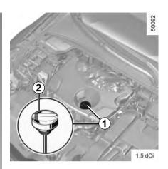
In order to prevent splashing, it is recommended that a funnel be used when topping up/filling the oil.
