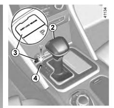
When setting off, if the lever is locked in position **P** even though you are pressing the brake pedal, the lever can be released manually. To do this, unclip the flap **3**, then insert a tool (with a hard rod to it) into the hole **4** and press the button **2** at the same time in order to unlock the lever.
