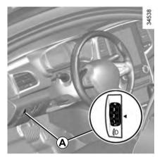
On vehicles fitted with this function, control **A** allows you to adjust the height of the beams according to the load.
