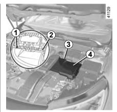
Lift the box cover 3 located behind the battery, then lift the battery half-cover 4.
