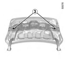
Replace the bulb 3. Bulb type: W16W.
