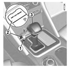
If the lever is stuck in **P**, even though you are depressing the brake pedal, the lever can be released manually.
