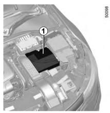
Battery 1 does not require any maintenance. You should not open it or add any fluid.
