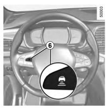
The cruising speed replaces the dashes and cruise control is confirmed by the appearance of the message "Adaptive cruise ctrl" and the indicator light "". If you try to activate the function below 31 mph (50 km/h) or above 86.8 mph (140 km/h), the message "Invalid speed" is displayed and the function will remain inactive.
