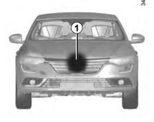
Using the sensor 1, this function notifies the driver about the time interval separating them from the vehicle in front, so they can respect a safe distance between the two vehicles.
