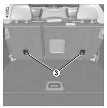
The third ring is located underneath the covers 2 or, depending on the vehicle, on the back of the rear seats 3. The rings are identified by the symbol.
