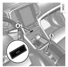
While driving, it is possible to leave the ECO mode temporarily in order to improve engine performance.
