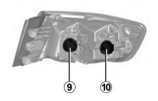
Refit the bulb holder and push the unit in fully until it locks in place.
