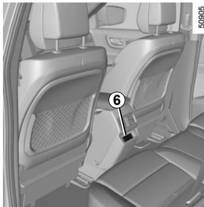
The sockets USB can also recharge accessories with a maximum power rating of 10.5 Watts (voltage: 5V) per socket, which have been approved by our Technical Department.
