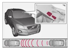
Laser sensor transmitter and receiver window<sup>16</sup>.
