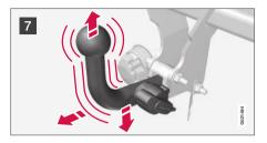
Check that the towball section is secure by pulling it up, down and back.
