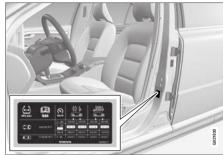
The tyre pressure label on the driver's side door pillar (between frame and rear door) shows which pressure the tyres should have at different loads and speed conditions. This is also specified in the tyre pressure table.
