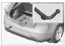
The detachable towbar must be stored in the foam block<sup>21</sup> under the cargo area floor when not in use.
