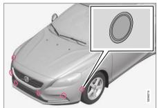
The PAP sensors are located in the bumpers<sup>44</sup> - 6 front and 4 rear.
