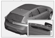
Rubber plate with electrical contact.
