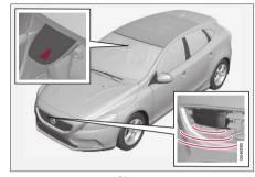
Camera and radar sensor<sup>24</sup>.
