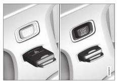
Ignition switch with remote control key extracted/inserted.
