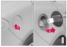
Open the fuel filler flap by slightly pressing in the rear part of the hatch.
