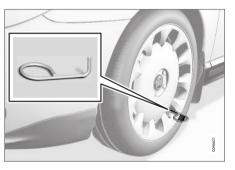
5. Screw together the towing eye with the wheel wrench\* to the stop position.
