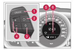
The steering wheel buttons and display in cars  $\mbox{\it without}$  speed limiter  $^6.$
