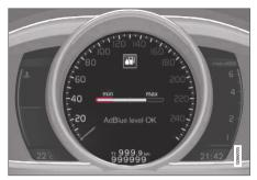
AdBlue level graphic: Each cursor represents approx. 25% of a full tank. When less than 25% of tank capacity remains, the amount of AdBlue that can be topped up is shown in litres.
