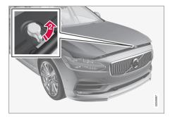
Turn the handle under the front edge of the hood counterclockwise to release it from the lock and lift.
