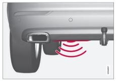
The foot movement sensor is located to the left of center under the rear bumper
