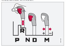
The gear selector can be moved back and forth freely between N and D. There is a mechanical shiftlock for the other positions.
