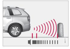
The system's rear sensors are activated automatically when the engine is started and are active if the vehicle rolls rearward with the gear selector in **N** or if **R** has been selected.
