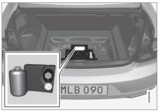
Location of the tire sealing system. Generic illustration - the appearance and location of the foam block may vary from model to model
