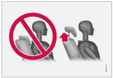
The center head restraint should be adjusted up or down according to the passenger's height. The restraint should be carefully adjusted to support the occupant's head.
