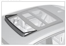
The laminated panoramic roof is equipped with a wind blocker that folds up when the roof is open.
