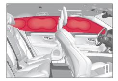
This system consists of inflatable curtains located along the sides of the roof liners, stretching from the center of both front side windows to the rear edge of the rear side door windows.
