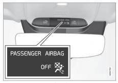
Occupant Weight Sensor (OWS) indicator light
