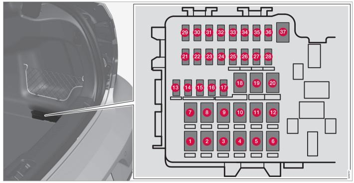
There is a fuse removal tool on the inside of the fuse box cover. There are also positions in the fuse box in the engine compartment for several extra fuses.
