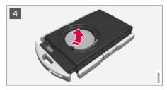
The battery's positive (+) side is up. Pry out the battery as shown in the illustration.
