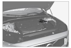
The support battery is located in a box next to the spring strut in the engine compartment
