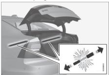
Preloaded springs for the power trunk release
