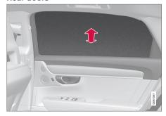
Each of the electrically operated sun curtains in the rear doors can either be fully opened or retracted.
