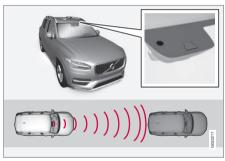
The camera and radar sensor monitor the distance to the vehicle ahead (generic illustration - certain details may vary from model to model)
