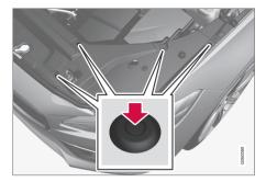
Release the pins in the plastic covering's four clips by pressing them down with a screwdriver or similar object and remove the covering.
