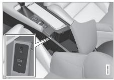
USB socket in the tunnel console
