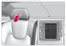
The outboard head restraints can be folded down in two ways from the center display.
