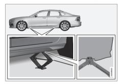
Raise the vehicle until the wheel to be changed is lifted off the ground. Remove the wheel holts.
