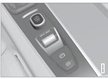
Start knob in the tunnel console between the front seats
