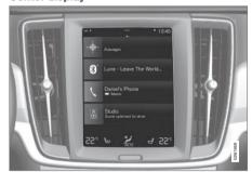
Many of the vehicle's main functions are controlled from the center display, a touchscreen that reacts to taps or other gestures. The number of physical buttons is thereby minimized. The screen can be operated with or without gloves.
