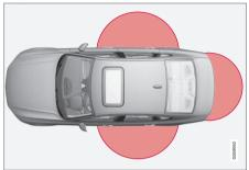
The shaded areas illustrate the range of the Passive Entry system's antennas
