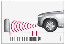
The system's front sensors are activated automatically when the engine is started and are active at speeds below approximately 6 mph (10 km/h).
