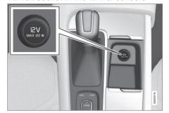
12-volt socket in the tunnel console for the front seats
