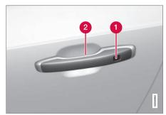
Outer indentation for locking, the pressure sensitive surface on the inside of the handle is for unlocking
