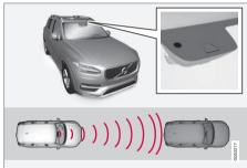
Location of the camera and radar sensor (generic illustration)
