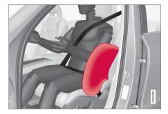
The SIPS airbag system is designed to help increase occupant protection in the event of certain side impact collisions. The SIPS airbags are designed to deploy only during certain side-impact collisions, depending on the crash severity, angle, speed and point of impact.
