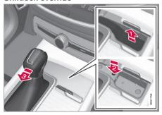
If the vehicle cannot be driven (e.g., due to a discharged battery), the shiftlock feature has to be overridden in order to move the gear selector
