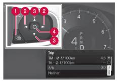
Use the right-side steering wheel keypad to navigate in the trip computer (generic illustration)
