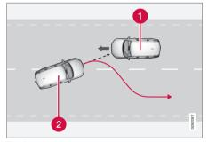
This function can provide steering assistance to help return the vehicle to its traffic lane
