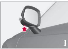
The side cameras are located in the respective door mirrors and show views along the sides of the vehicle.
