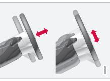
The steering wheel's height and reach can be adjusted
