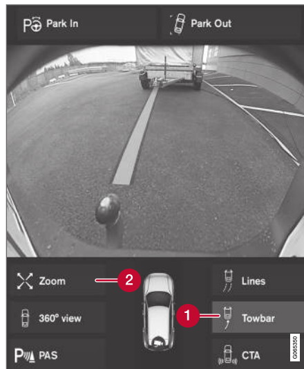
Towbar with trajectory line 114 .
