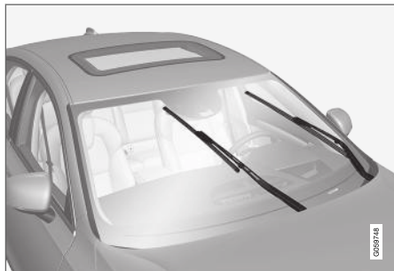
Windshield wipers in the service position.
