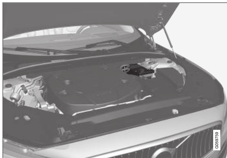
The support battery is located in a box next to the spring strut in the engine compartment.
