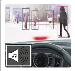
The optional system Collision Warning with Full Auto-brake and Pedestrian Detection has a feature that helps detect pedestrians and applies the brakes to help slow or stop the vehicle.
