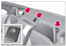
Your Volvo is equipped with child restraint top tether anchorages in the rear seat. They are located on the rear parcel shelf.
