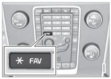
The \* **FAV** button can be used to store frequently used functions, making it possible to start the stored function by simply pressing \* **FAV**. One favorite (for example, **Equalizer**) can be programmed for each of the following infotainment system functions:
