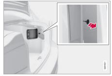
If necessary, the fuel filler door can be opened manually:
