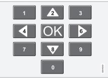
Buttons in the center console control panel, shown in the illustration, are used to navigate in a DVD's menus.
