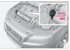
Check the level frequently. The fluid does not require changing. The fluid level must be between the **MIN** and **MAX** marks. For capacities and recommended fluid grade, see page 362.
