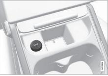
12-volt socket in the front tunnel console
