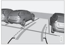
The lines on the screen are projected as if they were a path on the ground behind the
