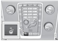
Button for steering wheel heating
