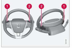
Steering-wheel mounted gear shift paddles
