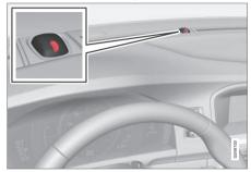
The status of the alarm system is indicated by the red indicator light on the dashboard (see illustration):
