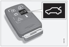
Trunk unlock button on the remote key
