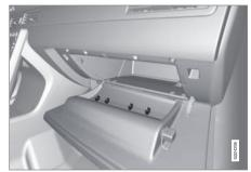
The owner's manual and maps can be kept here. There are also holders for pens and fuel cards. The glove compartment can be locked manually with the key blade, see page 68.
