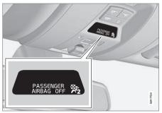
Occupant Weight Sensor (OWS) indicator light
