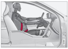
The seat belt should always be worn during pregnancy. But it is crucial that it be worn in the correct way. The diagonal section should wrap over the shoulder then be routed between the breasts and to the side of the belly. The lap section should lay flat over the thighs and as low as possible under the belly. It must never be allowed to ride upward. Remove all slack from the belt and ensure that it fits close to the body without any twists.
