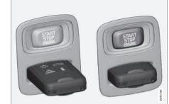
Ignition slot with remote key and **START/STOP ENGINE** button.
