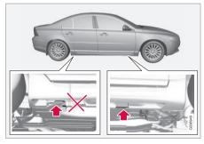
If a garage jack is used to lift the vehicle, the two jack attachments points should be used.
