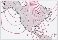
The earth is divided into 15 magnetic zones. The correct zone must be selected for the compass to work correctly.
