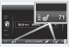
The current seat temperature setting is shown in the center console display
