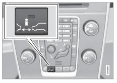
Press the button in the center instrument panel to switch this function on or off. The indicator light in the button illuminates when the function is on. Depending on the optional equipment selected, there may not be room for a Distance Alert button in the center console. In this case, the function is controlled through the menu system. Press **MY CAR** and go to **Settings**  $\rightarrow$  **Car settings**  $\rightarrow$  **Distance alert**  $\rightarrow$  **On/Off**.
