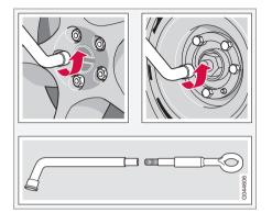
With the vehicle still on the ground, use the lug wrench/towing eyelet to loosen the wheel nuts ½ – 1 turn by exerting downward (counterclockwise) pressure.
