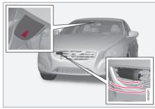
Camera and radar sensor<sup>1</sup>.
