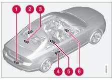
The keyless drive system has a number of antennas located at various points in the vehicle.
