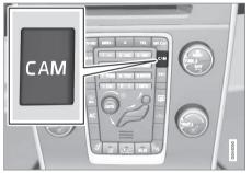
PAC is activated when the gear selector is moved to **R** if the system is selected in the **MY CAR** menu system or by pressing the **CAM** button in the center console. See page 193 for a description of the menu system.
