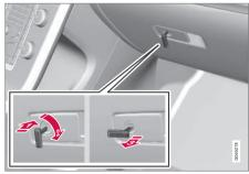
The glove compartment can only be locked and unlocked using the detachable key blade
