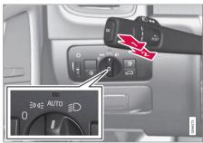
Headlight switch and steering wheel lever
