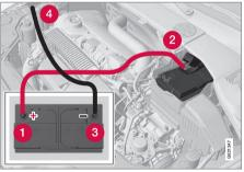
Connecting the jumper cables
