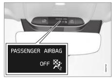
Occupant Weight Sensor (OWS) indicator light
