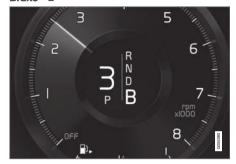
From the **B** position, it is possible to manually shift down to lower gears. **B** can be selected at any time while driving. When the accelerator pedal is released, the electric motor brakes the vehicle and the hybrid battery is recharged at the same time. This offers additional opportunities to recharge the hybrid battery, since the battery is charged even when the brake pedal is not depressed.
