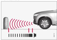
The warning signal has a continuous tone when the obstacle is less than approx.  $30\ \text{cm}$  (1 ft) from the vehicle.
