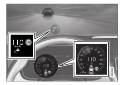
The previous illustration shows that Adaptive Cruise Control is set to maintain a speed of 110 km/h (68 mph) and is following a target vehicle ahead, which is traveling at the same speed.
