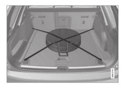
The spare wheel is stored in a bag and should be secured with two straps onto the floor of the trunk/cargo compartment when the vehicle is being driven. The straps should be strapped down crosswise over the wheel, attached to the load anchoring eyelets and pulled taut.
