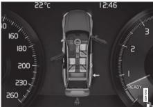
Graphics in the instrument panel with various types of warnings. The warning colors for the doors/trunk lid vary depending on the vehicle's speed.
