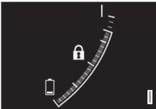
The symbol in the hybrid battery gauge indicates that the **Hold** function is activated. The
