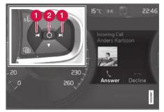
Examples of messages in the instrument panel and the right-side steering wheel keypad.
