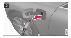
Open the charger door. Push the charging handle all the way into the vehicle's socket.
