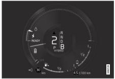
The vehicle generates electrical current to charge the battery, e.g. when the driver lightly presses the brake pedal or when engine braking is used on downgrades.
