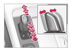
Select gears by moving the spring-loaded, non-locking gear selector forward or backward.
