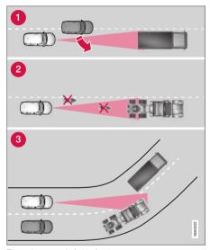
The radar sensor's field of vision.
