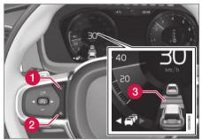
Controls for setting a time interval.
