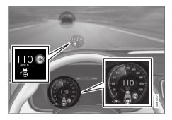
The previous illustration<sup>34</sup> shows that Pilot Assist is set to maintain a speed of 110 km/h (68 mph) and is following a target vehicle ahead that is traveling at the same speed.
