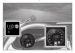
The previous illustration shows that Adaptive Cruise Control is set to maintain a speed of 110 km/h (68 mph) and that there is no target vehicle ahead to follow.
