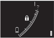
The first symbol is displayed in the hybrid battery gauge when Hold is activated.
