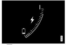
The <u>5</u> symbol is displayed in the hybrid battery gauge when Charge is activated.
