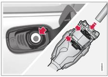
It is important to insert the pump's nozzle past both of the two flaps in the fuel filler pipe before beginning fueling. Instructions for fueling:
