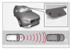
Location of the camera and radar sensor.
