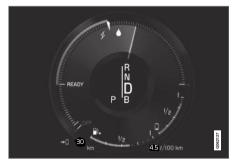
The electric motor cannot supply the requested power and the internal combustion engine will start.
