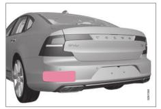
Location of rear radar sensors. Keep the marked area clean (on both the left and right sides of the vehicle).
