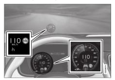
The previous illustration<sup>34</sup> shows that Pilot Assist is set to maintain a speed of 110 km/h (68 mph) and that there is no target vehicle ahead to follow.
