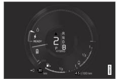
When the battery is being charged with the electric motor braking function, this will be indicated in the instrument panel. This function is active at speeds in the range of 150-5 km/h (93-3 mph). When braking at speeds outside of this range, or during harder braking, the hydraulic braking system is used to augment braking. This is indicated in the instrument panel with the pointer down in the red area.
