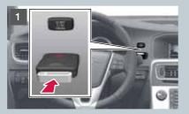
1. Holding the end of the remote key with the base of the key blade, insert the remote key into the ignition slot and press it in as far as possible.
