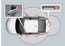
On keyless drive vehicles, it is only necessary to have a remote key in your possession to operate the central locking system and start the engine.
