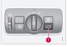
Press the button on the lighting panel (1) to unlock and pop open the trunk
