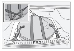
Turn the handle on the spare wheel bag in toward the rear seat. Secure the stitched strap hooks in the loading eyelets. Secure the long strap in one of the loading eyelets, wrap the strap around the spare wheel and through the lower handle. Secure the short strap on the long strap. Secure in the other loading eyelet and tighten.
