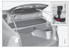
The vehicle is equipped with a florescent handle on the inside of the trunk lid, which can be used in an emergency situation to open the trunk from the inside. Pull the handle down to release the trunk lid. After use, the handle must be pushed back into its original position before the trunk can be closed.
