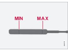
The oil level must be between the **MIN** and **MAX** marks on the dipstick
