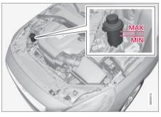
Check the level frequently. The fluid does not require changing. The fluid level must be between the **MIN** and **MAX** marks. For capacities and recommended fluid grade, see page 388.
