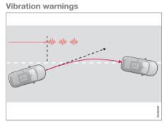
LKA provides vibrations in the steering wheel and steering assistance<sup>4</sup>.
