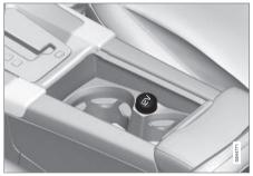
12-volt socket in the front tunnel console
