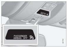
Occupant Weight Sensor (OWS) indicator light
