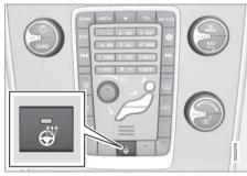
Button for steering wheel heating
