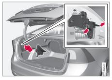
The bulbs in the taillight cluster are replaced from inside the trunk (not the LED functions).
