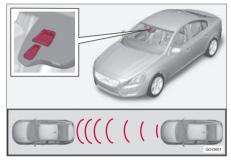
Location of the laser sensor in the windshield<sup>2</sup>
