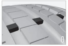
The tires have wear indicator strips running across or parallel to the tread. The letters **TWI** are printed on the side of the tire. When approximately 1/16" (1.6 mm) is left on the tread, these strips become visible and indicate that the tire should be replaced. Tires
