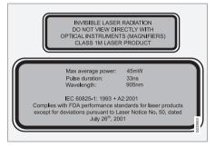
The upper decal describes the laser beam's classification and contains the following text:
