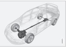
Your Volvo can be equipped with permanent All Wheel Drive, which means that power is distributed automatically between the front and rear wheels. Under normal driving conditions, most of the engine's power is directed to the front wheels. However, if there is any tendency for the front wheels to spin, an electronically controlled coupling distributes power to the wheels that have the best traction.
