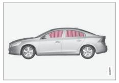
This system consists of inflatable curtains located along the sides of the roof liners, stretching from the center of both front side windows to the rear edge of the rear side door windows. It is designed to help protect the heads of the occupants of the front seats and the occupant of the outboard rear seating positions in certain side impact collisions.
