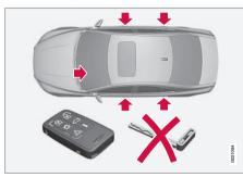
Locking/unlocking points with valet locking activated
