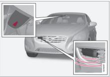
Camera and radar sensor<sup>1</sup>
