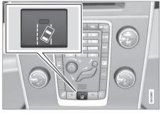
LDW can be switched on or off by pressing the button on the center console. A light in the button illuminates when the function is on. This is supplemented by graphic displays in the instrument panel, for example:
