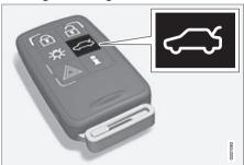
Trunk unlock button on the remote key
