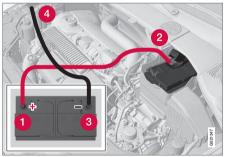
Connecting the jumper cables
