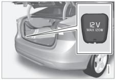
Fold down the cover to access the electrical socket.
