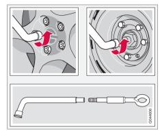
With the vehicle still on the ground, use the lug wrench/towing eyelet to loosen the wheel nuts ½ – 1 turn by exerting downward (counterclockwise) pressure.
