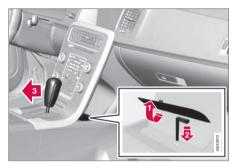
If the vehicle cannot be driven, for example because of a dead battery, the gear selector must be moved from the  $\mathbf{P}$  position before the vehicle can be moved<sup>4</sup>.
