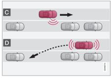
When the vehicle is backing up, PAP will steer it into the parking space.
