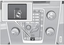
LKA can be switched on or off by pressing the button on the center console. A light in the button illuminates when the function is on.
