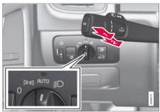
Headlight switch and steering wheel lever
