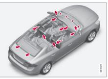
The incoming air is distributed from a number of different vents in the passenger compartment.
