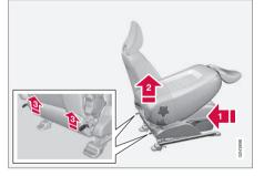
The front passenger seat backrest can be folded to a horizontal position to make room for a long load. Fold the backrest as follows:
