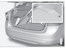
The load anchoring eyelets on both sides of the vehicle are used to fasten straps, etc., to help anchor items in the trunk.
