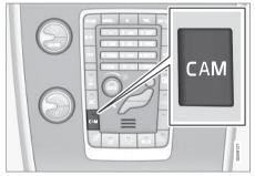
PAC is activated when the gear selector is moved to **R** if the system is selected in the MY CAR menu system or by pressing the **CAM** button in the center console. See page 215 for a description of the menu system.
