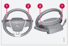
Steering-wheel mounted gear shift paddles
