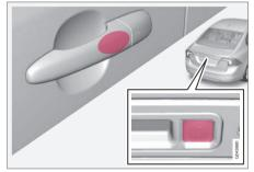
The touch-sensitive area on the outer door handles and a rubberised button next to the boot lid's rubberised pressure plate.
