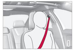
Correctly fitted seatbelt.
