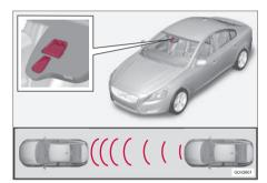
Laser sensor transmitter and receiver window<sup>13</sup>.
