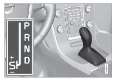
**D**: Automatic gear positions. +/-: Manual gear positions. **S**: Sport mode\*.
