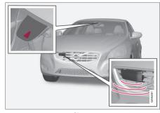
Camera and radar sensor<sup>21</sup>.
