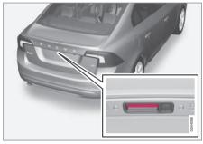
Rubber plate with electrical contact.
