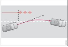
Warning with steering wheel vibration<sup>27</sup>.
