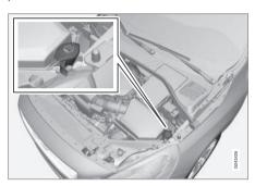
Topping up the washer fluid takes place by opening the blue cap.
