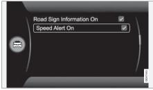
The driver can opt to receive a warning when the applicable speed limit is exceeded by 5 km/h (5 mph) or more. This warning is given by the symbol showing the applicable maximum speed temporarily flashing when this speed is exceeded. The function can be activated/deactivated in the menu system MY CAR. For a description of the menu system, see MY CAR (p. 109).
