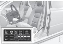
The tyre pressure label on the driver's side door pillar (between frame and rear door) shows which pressures the tyres should have at different loads and speed conditions. This is also specified in the tyre pressure table, see Tyres - approved tyre pressures (p. 436).
