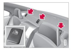
For cars with folding head restraints on the outside seats the head restraints should be folded to facilitate installation.
