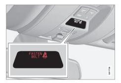
The audio reminder is speed dependent, and in some cases time dependent. The visual reminder is located in the roof console and in the combined instrument panel (p. 62).
