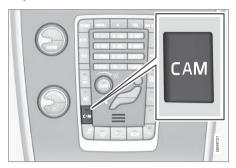
Press CAM - the screen shows the current camera view.
