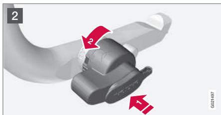
2 Premere la manopola di bloccaggio
