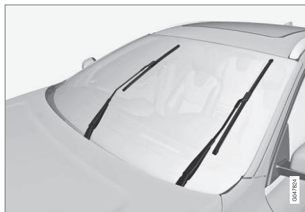
Wiper blades in service position
