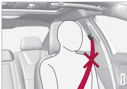
Incorrect height adjustment
