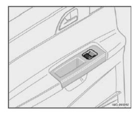
The rear door windows can be operated with the control on each door and with the switch on the driver's door.
