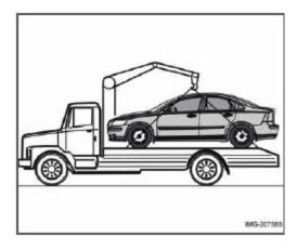
Volvo recommends the use of flat bed equipment for towing vehicles with front wheel drive. If wheel lift equipment must be used, please use extreme caution to help avoid damage to the vehicle.
