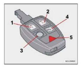
1. **Lock** - Press the Lock button on the remote once to lock all doors and the trunk. The turn signals will flash once to confirm locking.
