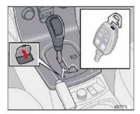
Shiftlock prevents the gear selector from being moved out of Park unless the ignition key is in position II and the brake pedal is depressed.
