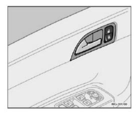
The switches near the door opening handles on the driver's and front passenger's doors can be used to lock or unlock all doors and the trunk, and to set the alarm.
