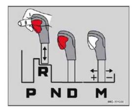
Depress the button on the front of the gear selector knob to move the selector between the R, N, D, and P positions.
