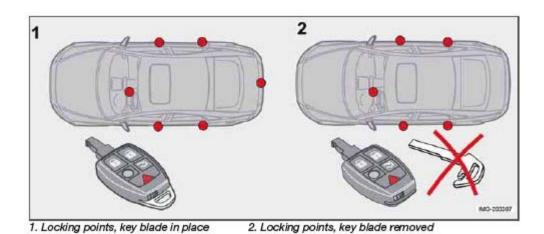
By utilizing the remote control with the key blade removed, the valet locking feature enables you to block access to the trunk and glove compartment for e.g. valet parking or when the car is brought to the retailer for service.
