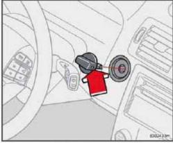
Removing the keyless drive start control
