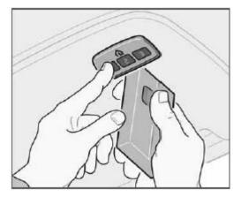
HomeLink<sup>1</sup> is a system that can be programmed to learn the codes of three different remote controlled-devices (for example, a garage door opener, remote lighting, entry gate). HomeLink's sun visor-mounted transceiver, powered by your car's electrical system, may then be used in place of your handheld remote controls. The HomeLink transceiver consists of three programmable buttons and an indicator light.
