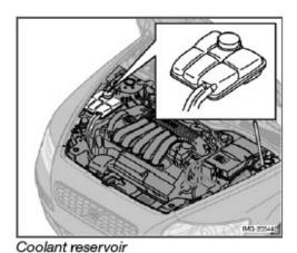
Normally, the coolant does not need to be changed. If the system must be drained, consult your Volvo retailer.
