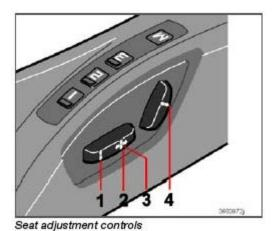
The power driver's seat can be adjusted:
