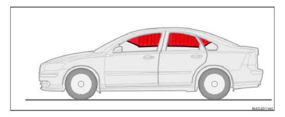
This system consists of inflatable curtains located along the sides of the roof liners, stretching from the center of both front side windows to the rear edge of the rear side door windows. It is designed to help protect the heads of the occupants of the front seats and the occupant of the outboard rear seating positions in certain side impact collisions.
