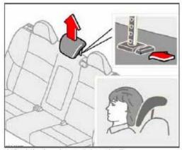
Adjust the head restraint vertically
