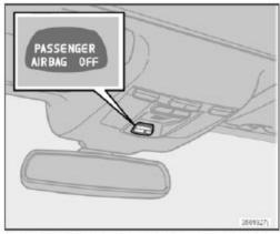
Occupant Weight Sensor (OWS) indicator light
