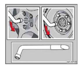
5. With the car still on the ground, use the lug wrench to loosen the wheel nuts 1/2 - 1 turn by exerting downward pressure. Turn the nuts counterclockwise to loosen.
