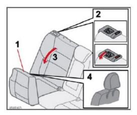
Both sections of the rear seat backrest can be folded down, together or separately, to enable you to transport long objects. Before folding down the rear seat backrests, the outboard seat belts can be attached to the clothes hook as shown in the center illustration. To fold down one or both sections:
