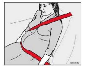
The seat belt should always be worn during pregnancy. But it is crucial that it be worn in the correct way. The diagonal section should wrap over the shoulder then be routed between the breasts and to the side of the belly. The lap section should lay flat over the thighs and as low as possible under the belly. It must never be allowed to ride upward. Remove all slack from the belt and insure that it fits close to the body without any twists.
