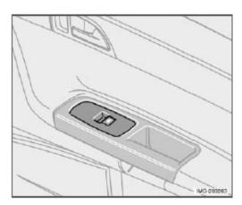
The control for the power window in the front passenger's door operates that window only.
