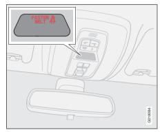
Unbelted occupants will be reminded to fasten their seatbelts through an audio and visual reminder. The audio reminder is speed dependent, and in some cases time dependent. The visual reminder is located in the roof console and the combined instrument panel.
