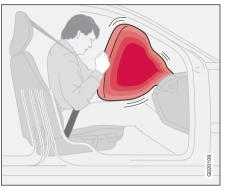
The car has an airbag<sup>1</sup> to supplement the protection afforded by the seatbelt on the passenger side. This airbag is folded up into a compartment above the glovebox, and its cover panel is marked **SRS AIRBAG**.
