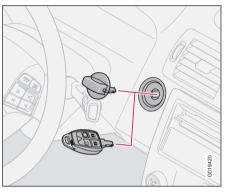
If the remote control battery is discharged then the Keyless Drive function does not work. In which case, start the car by using the remote control as ignition dial.
