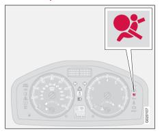
The airbag system<sup>1</sup> is continually monitored by the system control module. The warning symbol in the combined instrument panel illuminates when the ignition key is turned to position **I**, **II** or **III**. The symbol goes out after approx. 6 seconds provided the airbag system<sup>1</sup> is working correctly.
