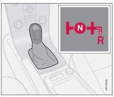
Only engage reverse gear when the car is stationary.
