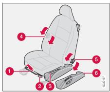
The driver's and passenger seats can be adjusted to the optimum sitting and driving positions
