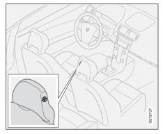
The coat hanger is located on the passenger seat head restraint. Only hang light garments on the hanger.
