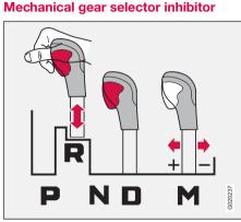
The gear selector can be moved forward and back freely between N and D. Other positions are locked with a latch that is released with the inhibitor button on the gear selector.
