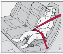
Volvo's integrated booster cushion for the outer rear seats is specially designed to provide optimum safety for children. Combined with the regular seatbelts, the booster cushion is approved for children weighing between 15 and 36 kg.
