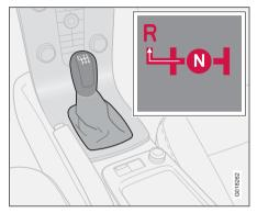
Only engage reverse gear when the car is stationary. Engage reverse gear by pressing down the gear lever and moving it to the left.
