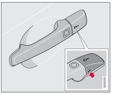
If central locking cannot be activated with the remote control, e.g. if the batteries are discharged, then the driver's door can be opened as follows:
