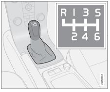
Depress the clutch pedal fully with each gear change. Remove your foot from the clutch pedal between gear changes! Follow the appropriate shifting pattern.
