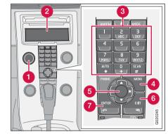
Infotainment is a system that integrates the audio system and the phone<sup>1</sup>. The infotainment system can be easily operated using the control panel or the steering wheel keypad<sup>1</sup>, see page 54. The display (2) shows messages and information on the current function.
