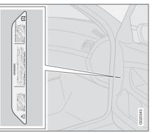
Location of airbag decal in door opening on front passenger side in left-hand drive cars.
