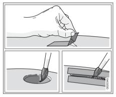
Before touching up paintwork, the car must be clean and dry and at a temperature above 15  $^\circ C.$
