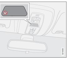
Indicator showing that the passenger airbag (SRS) is activated.
