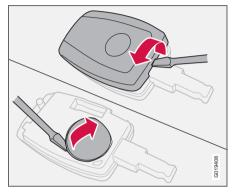
If the locks repeatedly fail to respond to signals from the remote control at a normal distance, the battery should be replaced (type CR 2450, 3 V).
