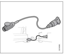
An adapter is required if the car's towbar has 13 pin electrics and the trailer has 7 pin electrics. Use an adapter cable approved by Volvo. Make sure the cable does not drag on the ground.
