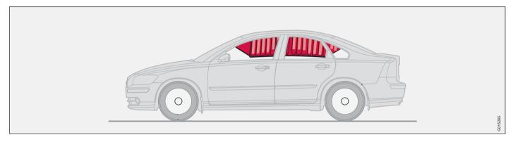
The inflatable curtain IC (Inflatable Curtain) is a supplement to the SIPS and the airbags. It is fitted in the headlining along both sides of the roof and protects all of the vehicle's outer seats. A sufficiently violent collision trips the sensors and the inflatable curtain is inflated. The inflatable curtain helps to prevent the driver and passengers from striking their heads on the inside of the car during a collision.
