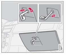
The owner's manual and maps can be kept here. There are also holders for coins, pens and fuel cards. The glovebox can be locked with the remote control's detachable key blade. For further information on the key blade, see page 99.
