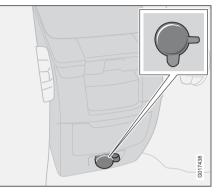
The electrical socket can be used for various accessories, such as mobile phone chargers and coolers.
