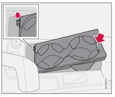
There is space for a double cup holder under the roller cover. The space can be used for storage by lifting out the cup holder. Lift at the rear edge of the cup holder where there is a recess.
