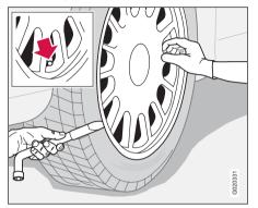
Set up the warning triangle if a wheel must be replaced at a busy location. Make sure that the car and jack are on a firm horizontal surface.
