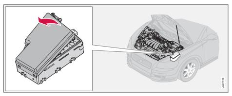
The fuse box has 36 fuse positions. Be sure to replace a blown fuse with a new fuse of the same colour and amperage.
