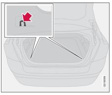
The load retaining eyelets are used to fasten straps or nets to anchor items in the cargo area.
