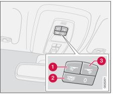
Passenger compartment lighting and reading lamps
