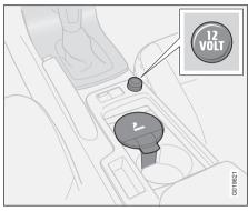
The electrical socket can be used for 12 V accessories, such as mobile phone chargers and coolers. The maximum current is 10 A. For the socket to supply current, the ignition key must be in at least position **I**.
