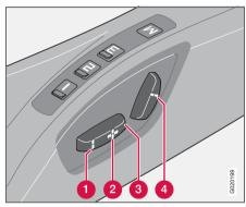
The seats can be adjusted for a certain time after unlocking the door with the remote control without the key being inserted into the ignition switch. The seat can always be set in ignition position I or II.
