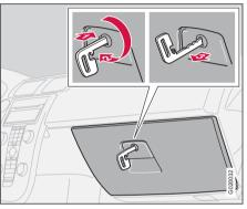
This function is intended for when the car is left for service, with a hotel parking valet or similar. The glovebox is then locked and the boot lid lock is disconnected from the central locking. The cargo area cannot be opened with either the central locking button in the front doors or the remote control.
