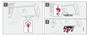
The fuse box has 50 fuse positions. The fuses are located under the glovebox. The box also provides space for several spare fuses. Tools for fuse replacement are located in the relay/fuse box in the engine compartment, see page 200.
