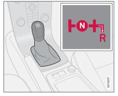
Only engage reverse gear when the car is stationary. To engage reverse gear, the gear lever must first be put in position  $\mathbf{N}$ . Reverse gear cannot therefore be engaged directly from fifth gear due to the reverse gear inhibitor.
