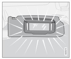
The light comes on automatically when the cover is lifted.
