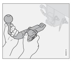
Turn the locking wheel down fully, until it comes to a stop. Hold it in this position while pulling the towball rearward and upward.
