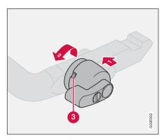
Check that the indicator window (3) shows red. If the window does not show red, press in (1) and turn the locking wheel anticlockwise (2) until you hear a click. O
