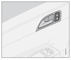
The doors and the boot lid can be locked or unlocked simultaneously using the lock button by the door handle.
