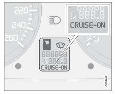
Increase or decrease the locked speed by pressing and holding + or -. The speed of the car when the button is released is set as the new speed.
