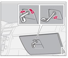
The glovebox can only be locked/unlocked using the remote control's detachable key blade. For information on removing the key blade, see page 99.
