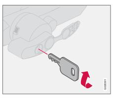
Ensure that the mechanism is in the unlocked position by turning the key clockwise.
