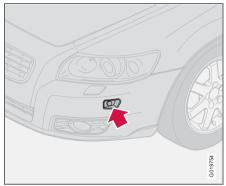
Connecting the engine block heater
