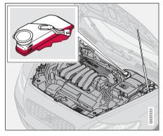
The brake and clutch fluid have a common reservoir<sup>1</sup>. The fluid level must be between the **MIN** and **MAX** marks. Check the level regularly. Change the brake fluid every other year or at every other regular service.
