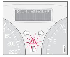
If the car is involved in a collision, the text **CRASH MODE - SEE MANUAL** may appear on the information display. This means that the car has reduced functionality. Crash mode is a protective state that is enforced when the collision may have damaged the car's vital functions, such as the fuel lines, sensors for one of the safety systems, or the brake system.
