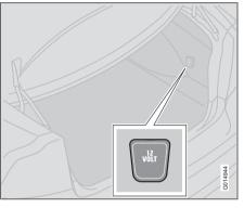
Fold down the cover to access the electrical socket. This socket works regardless of whether or not the ignition is on.
