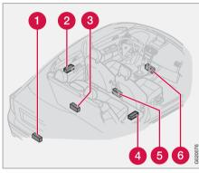
The keyless drive system has a number of antennas located at various points in the vehicle.
