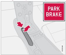
The parking brake lever is located between the front seats.
