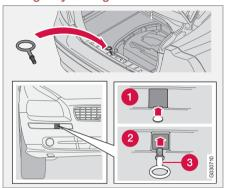
The towing evelet is located under the floor of the trunk. This eyelet must be screwed into the positions provided on the right sides of either the front or rear bumper (see the illustration).
