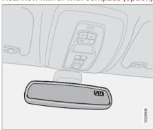
The upper right-hand corner of the rearview mirror has an integrated display that shows the compass direction toward which the car is pointing. Eight different directions can be displayed: N, NE, E, SE, S, SW, W and NW. The display shows your car's orientation with respect to true north.
