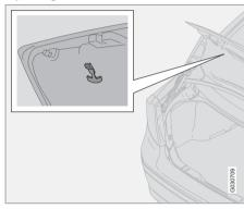
The vehicle is equipped with a florescent handle on the inside of the trunk lid, which can be used in an emergency situation to open the trunk from the inside.
