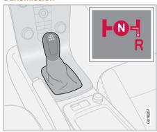
Reverse gear should only be engaged from a complete stop.
