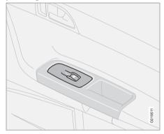
The control for the power window in the front passenger's door operates that window only.
