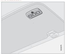
The HomeLink Wireless Control System provides a convenient way to replace up to three hand-held radio-frequency (RF) transmitters used to activate devices such as gate operators, garage door openers, entry door locks, security systems, even home lighting. Additional HomeLink information can be found on the Internet at www.homelink.com.
