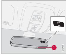
The earth is divided into 15 magnetic zones. The compass is initially set for the zone to which the car was delivered, and should always be adjusted if the car is driven to a new magnetic zone. A "C" will be displayed if calibration becomes necessary.
