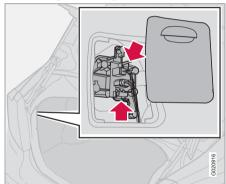
All bulbs in the taillight cluster can be replaced from the trunk. To access the bulb holders:
