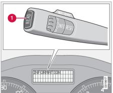
When an indicator or warning light in the instrument panel comes on, a message is also shown in the information display. To read a message:
