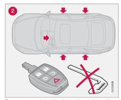
Remote control: Locking/unlocking points with key blade removed (with valet locking activated)
