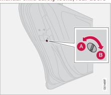
The controls are located on the rear inside edges of the doors, and are only accessible when the doors are open.
