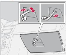
The glove compartment can only be locked and unlocked using the detachable key blade on the remote control, see page 120 for information on removing the key blade from the remote control.
