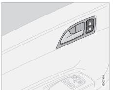
The switches near the door opening handles on the driver's and front passenger's doors can be used to lock or unlock all doors and the trunk, open the side windows<sup>1</sup>, and to set the alarm.
