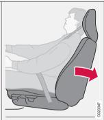
The WHIPS system consists of specially designed hinges and brackets on the front seat backrests designed to help absorb some of the energy generated in a collision from the rear (when the vehicle is "rearended").
