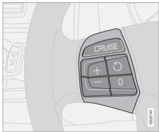
The cruise control buttons are located on the left side of the steering wheel hub.
