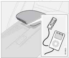
An auxiliary device, such as an iPod, MP3 player or a USB flash drive can be connected to the audio system via the connector in the center console storage compartment. A standard cable from an iPod or MP3 player can be routed under the cover to the AUX connector in the storage compartment.
