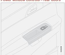
The rear door windows can be operated with the control on each door and with the switch on the driver's door.
