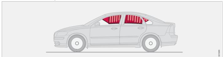
This system consists of inflatable curtains located along the sides of the roof liners, stretching from the center of both front side windows to the rear edge of the rear side door windows. It is designed to help protect the heads of the occupants of the front seats and the occupant of the outboard rear seating positions in certain side impact collisions.
