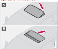
To operate the moonroof, the ignition key must first be turned to the intermediate or drive position (position I, II or the engine running). The moonroof can be opened in two ways:
