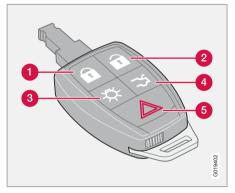
Lock – Press the Lock button on the remote once to lock all doors and the trunk. The turn signals will flash once to confirm locking.
