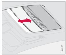
The optional moonroof features a sliding visor. The visor slides open automatically when the moonroof is opened, and must be closed manually.
