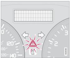
If the vehicle has been involved in a collision, the text **CRASH MODE SEE MANUAL** may appear in the information display. This indicates that the vehicle's functionality has been reduced.
