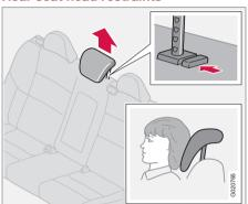
Adjust the head restraint vertically
