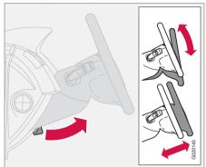
Both the height and the reach of the steering wheel can be adjusted to a comfortable position for the driver.
