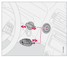
Removing the keyless drive start control
