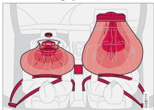
The front airbags supplement the three-point seat belts. For these airbags to provide the protection intended, seat belts must be worn at all times.
