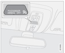
Occupant Weight Sensor (OWS) indicator light
