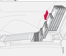
The deep storage compartment has room for 10 CD jewel cases. These cases must be inserted with their spines upward in order to allow space for 10 cases in the storage compartment
