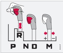
Depress the button on the front of the gear selector knob to move the selector between the **R**, **N**, **D**, and **P** positions.
