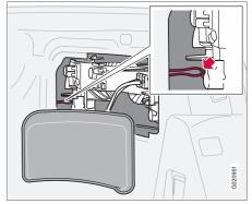
If it should be necessary to manually unlock the fuel filler door from the trunk, the power retractable hard top should be up.
