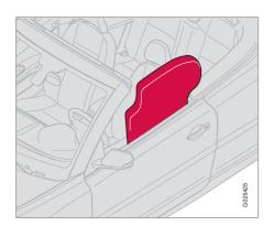
The DMIC is a supplement to the structural side impact protection. These inflatable curtains are concealed in the upper section of both doors.
