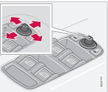
The mirror control switches are located on the driver's door armrest.
