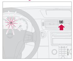
The four-way flasher should be used to indicate that the vehicle has become a traffic hazard.
