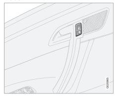
The switches near the door opening handles on either door can be used to lock or unlock both doors and the trunk, and to set the alarm.
