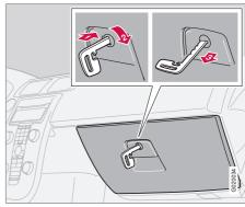
The glove compartment can only be locked and unlocked using the detachable key blade on the remote key, see page 119 for information on removing the key blade from the remote key.
