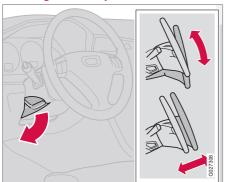
Both the height and the reach of the steering wheel can be adjusted to a comfortable position for the driver.
