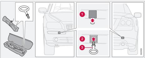
The towing eyelet is located in the tool bag, which is stowed in the ski hatch. This eyelet must be screwed into the positions provided on the right sides of either the front or rear bumper (see the illustration).
