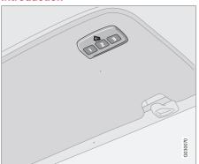
The HomeLink¹ Wireless Control System provides a convenient way to replace up to three hand-held radio-frequency (RF) transmitters used to activate devices such as gate operators, garage door openers, entry door locks, security systems, even home lighting. Additional HomeLink information can be found on the Internet at www.homelink.com.
