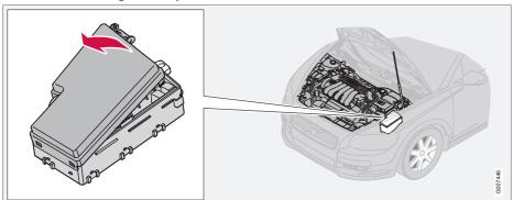
The fuse box in the engine compartment has positions for 36 fuses.
