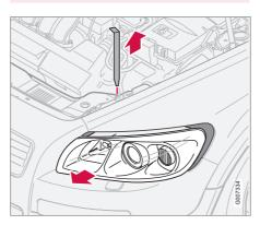
The entire headlight housing must be lifted out when replacing the high/low beam, parking
