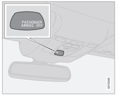
Occupant Weight Sensor (OWS) indicator light
