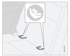
Lower anchors for ISOFIX-equipped child seats are located in both rear seating positions, hidden below the backrest cushions. Symbols on the seat back upholstery mark the anchor positions (see the illustration).
