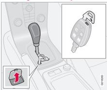
Shiftlock prevents the gear selector from being moved out of the **P**position unless the ignition key is in position **II** and the brake pedal is depressed.
