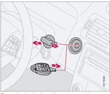
Removing the keyless drive start control
