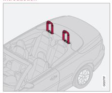
Deployed ROPS roll bars
