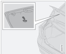
The vehicle is equipped with a florescent handle on the inside of the trunk lid, which can be used in an emergency situation to open the trunk from the inside.
