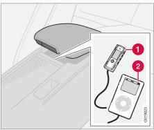
An auxiliary device, such as an iPod®, MP3 player or a USB flash drive can be connected to the audio system via the connector in the center console storage compartment. A standard cable from an iPod® or MP3 player can be routed under the cover to the AUX connector in the storage compartment.
