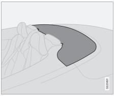
When lowered, the power retractable hard top is concealed by a cover, see the illustration.
