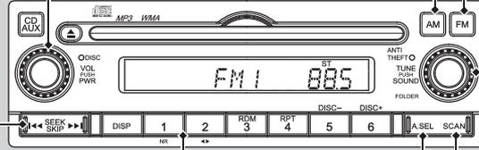
The diagram shows a car stereo control panel with various buttons and a digital display. The display shows 'FM1 88.5' and 'ST'. Callouts point to the following features: 'VOL/PWR' knob, 'SEEK/SKIP' buttons, 'DISP' button, '1-6' preset buttons, 'A.SEL' button, 'SCAN' button, 'AM/FM' buttons, and 'TUNE/SOUND' knob. The stereo also has a 'CD AUX' slot, 'MP3 WMA' indicator, and 'ANTI THEFT O TUNE FOLDER' label.
