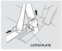
When you are folding the rear center seat-back, use the latch plate to release the center seat belt from the detachable anchor (see page 109). Allow the seat belt to retract into the holder on the ceiling and store the buckles in it.
