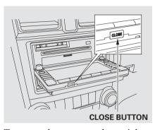
To return the screen to the upright position, press the CLOSE button on the edge of the screen panel. Do not use the folded down screen as a tray. If you put a cup, for example, on the screen, the liquid inside the cup may spill on the screen when you go over a bump.
