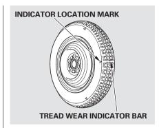
Replace the tire when you can see the tread wear indicator bars. The replacement tire should be the same size and design, mounted on the same wheel. The spare tire is not designed to be mounted on a regular wheel, and the spare wheel is not designed for mounting a regular tire. If you have a flat tire while driving, stop in a safe place to change it. Drive slowly along the shoulder until you get to an exit or an area to stop that is far away from the traffic lanes.
