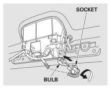
4. Pull the bulb straight out of its socket. Push the new bulb straight into the socket until it bottoms.
