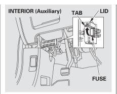
The auxiliary fuse box is located next to the interior fuse box.
