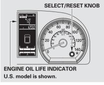
To see the current engine oil life, turn the ignition switch to the ON (II) position, then press and release the select/reset knob repeatedly until the engine oil life indicator appears (see page 69).
