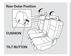
To pivot the outer head restraint down for better visibility, press the tilt button on the side of the head restraint. It folds down forward. To raise the head restraint, pivot it up by hand. Make sure the head restraint locks in position.
