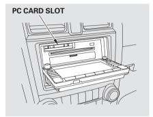
The PC card slot is behind the navigation screen. To use the PC card player, press the OPEN button beside the screen. The screen folds back, and the PC card slot appears.
