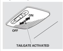
The cargo area light has a three-position switch. In the OFF position, the light does not come on. In the center position, it comes on when you open the tailgate. In the ON position, it stays on continuously.
