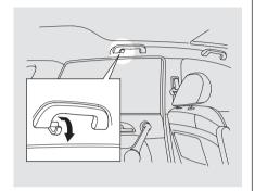
To use a coat hook, slide it out slightly, then pull it down.
