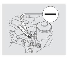
4. Connect the second jumper cable to the negative (—) terminal on the booster battery. Connect the other end to the stud bolt on the engine side as shown. Do not connect this jumper cable to any other part of the engine.
