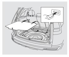
3. Open the tailgate. Raise the cargo area floor lid by lifting up with the strap, and remove it from cargo area by disengaging the tabs.
