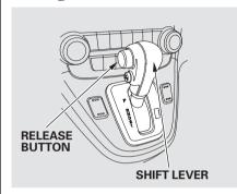
To shift from any position, press firmly on the brake pedal and the release button on the side of the shift lever. You cannot shift out of Park when the ignition switch is in the LOCK (0) or ACCESSORY (I) position.
