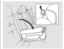
The rear center seat-back has a cargo area pass-through. To use the cargo area pass-through, pull up the release on top of the center seat-back and fold it down.
