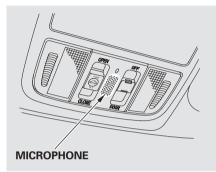
• Air or wind noise from the dashboard and side vents and all windows may interfere with the microphone. Adjust or close them as necessary.
