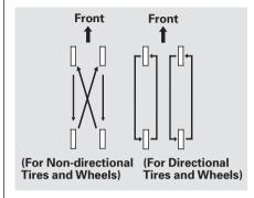
To help increase tire life and distribute wear more evenly, rotate the tires according to the maintenance messages displayed on the information display. Move the tires to the positions shown in the diagram each time they are rotated. If you purchase directional tires, rotate only front-to-back. When the tires are rotated, make
