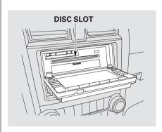
Insert a disc about halfway into the disc slot. The drive will pull the disc in the rest of the way and begin to play it.
