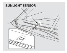
The climate control system has two sensors: a sunlight sensor on top of the dashboard, and a temperature sensor next to the steering column. Do not cover the sensors or spill any liquid on them.
