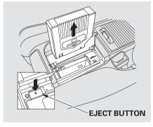
2. Push the EJECT button to remove the CD magazine. The magazine will pop up automatically.
