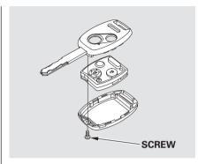
1. Remove the screw at the base of the transmitter with a small Phillips-head screwdriver.
