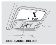
To open the sunglasses holder, push then release the raised detent. It will unlatch and swing down. To close it, push it until it latches. Make sure the holder is closed while you are driving.
