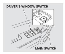
Turn the ignition switch to the ON (II) position to raise or lower any window. To open the window, push the switch down and hold it. Release the switch when you want to stop the window. To close the window, pull back on the switch and hold it.
