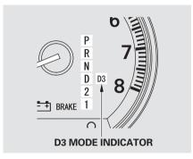
When the D3 mode is on, the transmission selects only the first three gears. Use D3 mode when towing a trailer, or to provide engine braking when going down a steep hill. D3 mode can also keep the transmission from cycling between third and fourth gears in stop-and-go driving.
