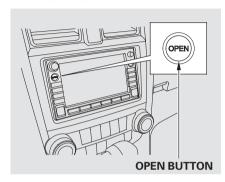
The in-dash disc player is behind the navigation screen. To use the disc player, press the OPEN button beside the screen. The screen folds back, and the disc slot appears.
