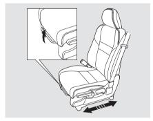
To adjust the seat forward or backward, pull up on the bar under the seat cushion's front edge. Move the seat to the desired position, and release the bar. Try to move the seat to make sure it is locked in position.
