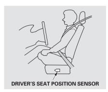
The driver's advanced front airbag system includes a seat position sensor under the seat. If the seat is too far forward, the airbag will inflate with less force, regardless of the severity of the impact.
