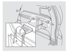
If equipped Your vehicle also has cargo hooks on the side panel in the cargo area. They are designed to hold light items. Heavy objects may damage the hook. Make sure any items put on each hook weigh less than 6.5 lbs (3 kg).
