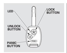
LOCK — Press this button once to lock all doors and the tailgate. Some exterior lights will flash once. When you push LOCK twice within 5 seconds, you will hear a beep to verify that the doors and the tailgate are locked and the security system (if equipped) has set. You cannot lock the doors and the tailgate if any door or the tailgate is not fully closed or the key is in the ignition switch.
