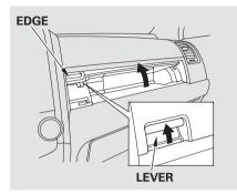
Open the upper glove box by pushing up the lever. Close it by pulling down on the edge under the lever.
