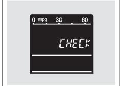
Your vehicle's onboard diagnostic system will detect a loose or missing fuel fill cap as an evaporative system leak. The first time a leak is detected a "CHECK FUEL CAP" message appears on the information display.
