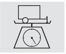
Total Trailer Weight: The maximum allowable weight of the trailer and everything in or on it must not exceed 1,500 lbs (680 kg). Towing a load that is too heavy can seriously affect your vehicle's handling and performance. It can also damage the engine and drivetrain.
