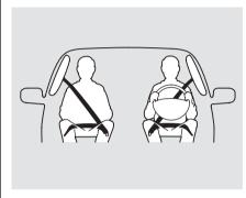
In addition, your vehicle has side curtain airbags to help protect the heads of the driver, front passenger, and passengers in the outer rear seating positions during a moderate to severe side impact or rollover (see page 31 for more information on how your side curtain airbags work).
