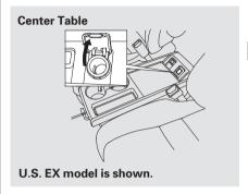
To use an accessory power socket, the ignition switch must be in the ACCESSORY (I) or ON (II) position.
