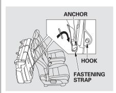
4. Pull out the fastening strap from the slit on the seat-back. Then attach the anchor on the fastening strap to the hook on the center pillar.
