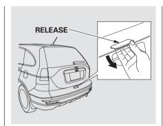
To open the tailgate, push the release, and lift up. To close the tailgate, use the tailgate handle to lower it, then press down on the back edge.
