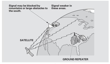
The XM satellites are in orbit over the equator; therefore, objects south of the vehicle may cause satellite reception interruptions. To help compensate for this, ground-based repeaters are placed in major metropolitan areas. Satellite signals are more likely to be blocked by tall buildings and mountains the farther north you travel from the equator. Carrying large items on a roof rack can also block the signal.
