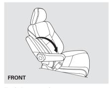
Each front seat has an armrest on the side of the seat-back. To use it, pivot it down.
