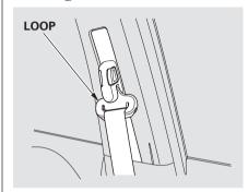
If your seat belts get dirty, use a soft brush with a mixture of mild soap and warm water to clean them. Do not use bleach, dye, or cleaning solvents. Let the belts air-dry before you use the vehicle. Dirt build-up in the loops of the seat belt anchors can cause the belts to retract slowly. Wipe the insides of the loops with a clean cloth dampened in mild soap and warm water or isopropyl alcohol.
