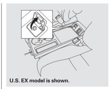
When a compatible audio unit is connected to the jack, press the AUX or CD/AUX button (AUX icon on models with navigation system) to select it.
