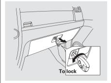
Open the lower glove box by pulling the bottom of the handle. Close it with a firm push. Lock or unlock the glove box with the master key.
