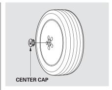
15. Remove the center cap before storing the flat tire.
