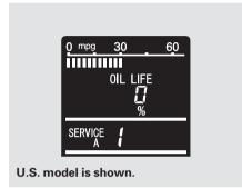
When the remaining engine oil life is 0 percent, the engine oil life indicator will blink. The display comes on every time you turn the ignition switch to the ON (II) position. The Maintenance Minder indicator ( ) also comes on and remains on in the instrument panel. When you see this message, immediately have the indicated maintenance done by your dealer.
