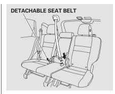
The lap/shoulder belt in the center seating position on the rear seat is equipped with a detachable seat belt that has two parts: a small latch plate and an anchor buckle.
