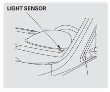
The automatic lighting feature is controlled by a sensor located on top of the dashboard. Do not cover this sensor or spill liquids on it. **Daytime Running Lights**
