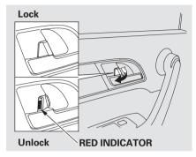
The lock tab on any passenger's door locks and unlocks that door.
