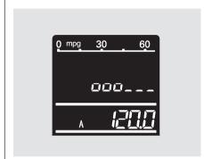
To reduce glare at night, the instrument panel illumination dims when you turn the light switch to ₹00₹ or ≣□ . Turning the select/reset knob fully to the right until you hear a beep will cancel the reduced brightness.
