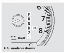
These indicators on the instrument panel show which position the shift lever is in. The "D" indicator comes on for a few seconds when you turn the ignition switch to the ON (II) position. If it flashes while driving (in any shift position), it indicates a possible problem in the transmission.
