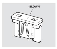
5. Look for a blown wire inside the fuse. If it is blown, replace it with one of the spare fuses of the same rating or lower.
