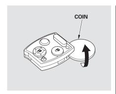
3. Inside the transmitter, separate the inner cover from the keypad by carefully prying on the edge with a coin.
