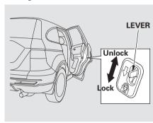
The childproof door locks are designed to prevent children seated in the rear from accidentally opening the rear doors. Each rear door has a lock lever near the edge. With the lever in the LOCK position (lever is down), the door cannot be opened from the inside regardless of the position of the lock tab. To open the door, push the lock tab forward and use the outside door handle.
