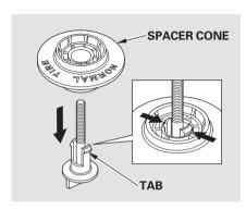
To remove the spacer cone, squeeze the tabs on the wing bolt to disengage it from the center of the spacer cone, then pull the bolt downward.
