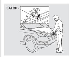
2. Reach in between the hood and the front grille with your fingers. The hood latch handle is above the "H" logo. Push this handle up until it releases the hood. Lift the hood.
