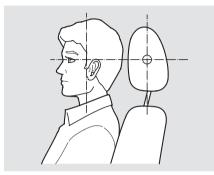
Adjust the driver's head restraint so the center of the back of your head rests against the center of the restraint.
