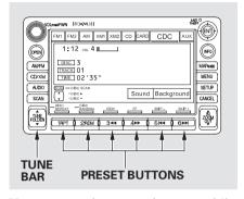
You can use the preset buttons while a disc is playing to select passages and change tracks. Each preset button function is shown on the bottom of the screen. **SKIP** — Push the ►►I button (preset 6) to play the next track on the disc. Push the I◄► button (preset 5) once to replay the track in play; press it twice to replay the previous track.
