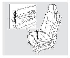
The height of your driver's seat is adjustable. To raise the seat, repeatedly pull up the lever on the outside of the seat cushion. To lower the seat, push the lever down repeatedly.
