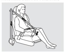
For added protection, the front seat belts are equipped with automatic seat belt tensioners. When activated, the tensioners immediately tighten the belts to help hold the driver and a front passenger in position. The tensioners can be activated during a collision in which the front airbags *do not deploy*. In this case, the airbags would not be needed, but the additional restraint could be helpful.
