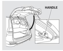
Keep the tailgate closed at all times while driving to avoid damaging the tailgate and to prevent exhaust gas from getting into the interior. See **Carbon Monoxide Hazard** on page 55.
