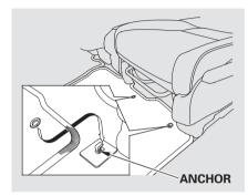
The floor mats that came with your vehicle hook over the floor mat anchors. This keeps the floor mats from sliding forward, possibly interfering with the pedals, or backwards, making the front passenger's weight sensors ineffective.
