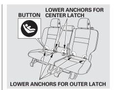
When you install a child seat in the rear center seating position, use the center lower anchors as shown in the illustration. To install a child seat in either outer seating position, use the outer lower anchors. You can install up to two child seats at a time using the outer lower anchors.
