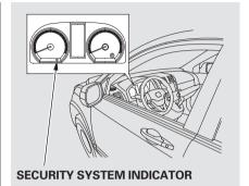
Once the security system is set, opening any door without using the key or the remote transmitter, the hood, or the tailgate will cause the system to alarm.
