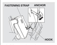
5. Pull down on the anchor to engage the upper part of the anchor securely on the hook, and make sure the seat is secure. Make sure that the folded up right rear seat does not interfere with the front passenger's seat-back. This will cause the front passenger's weight sensors and the front passenger's seat belt reminder indicator to work improperly (see page 33). Also check the passenger airbag off indicator to assure proper operation of the passenger's advanced front airbag.
