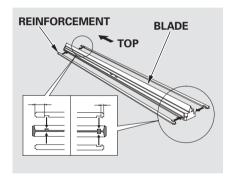
Make sure the three rubber tabs inside the blade fit to each notch of the reinforcement, as shown.
