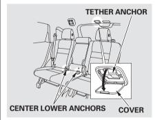
To install a LATCH-compatible child seat in the rear center seating position, use the center lower anchors as shown above.
