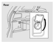
Make sure to put the socket cover back in place to prevent any small foreign objects from getting into the socket.
