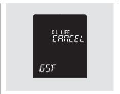
To adjust the outside temperature display, press and hold the select/reset knob for 10 seconds. The display changes as shown above. Select the outside temperature indicator by turning the select/reset knob. The display begins to blink. Push the same knob to enter this setting, then turn it to adjust the temperature. The following sequence will appear for each: 0, 1, 2, 3, 4, 5, -5, -4, -3, -2, -1, 0 (U.S.) or 0, 1, 2, 3, -3, -2, -1, 0 (Canada).
