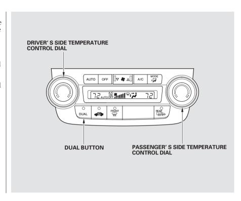
To set the driver's side temperature to a different value than the passenger's side, press the DUAL button, then turn the temperature control dial on the control panel. To set the passenger's side to a different value than the driver's side, turn the passenger's side temperature control dial. You can adjust the passenger's side without pressing the DUAL button first.
