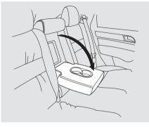
On vehicles with rear seat armrest The rear seat also has a beverage holder in the center armrest. To use it, pivot the armrest down.
