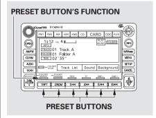
You can use the preset buttons while a card is playing to select or change files. Each preset button's function is shown on the bottom of the screen.
