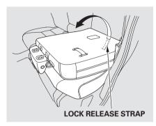
3. Unlock the seat from the floor by pulling the lock release strap located at the rear of the seat cushion, under the seat back, then lift the rear of the seat.
