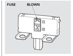
3. Check each of the large fuses in the under-hood fuse box by looking through the side window at the wire inside. Removing these fuses requires a Phillips-head screwdriver.
