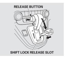
6. Remove the key from the shift lock release slot, then reinstall the cover. Make sure the notch on the cover is on the right side. Insert the key into the ignition switch, press the brake pedal, and restart the engine.
