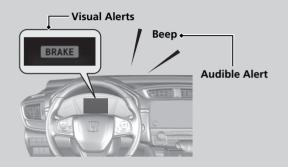
At system's earliest collision alert stage, you can change the distance (**Long/Normal/Short**) between vehicles at which alerts will come on through audio/information screen\* setting options.
