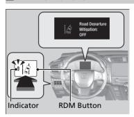
Press the RDM button to turn the system on and off.
