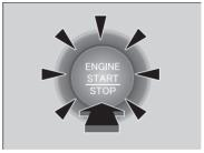
Touch the center of the ENGINE START/ STOP button with the H logo on the smart entry remote while the ENGINE START/ STOP button is flashing.
