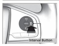
Press the (Interval) button to change the ACC with LSF following-interval. Each time you press the button, the following-interval (the interval behind a vehicle detected ahead of you) setting cycles through extra long, long, middle, and short following-interval.
