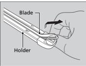
**4.** Pull the wiper blade in the opposite direction to slide it out of the holder.
