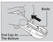
**3.** Pull the end of the wiper blade to the direction of the arrow in the image until it unfastens from the holder's end cap.
