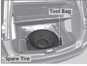
**2.** Take the tool bag out of the cargo area. Take the wheel nut wrench and jack handle bar out of the tool bag.
