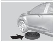
**6.** Place the compact spare tire under the vehicle body (wheel side up) near the tire that needs to be replaced.
