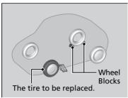
**5.** Place a wheel block or rock in the front and rear of the wheel diagonal to the flat tire.
