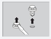
Insert the clip with the center pin raised, and push until it is flat.
