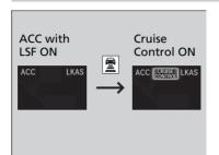
Press and hold the (interval) button for one second. **Cruise Mode Selected** appears on the driver information interface for two seconds, and then the mode switches to Cruise.
