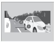
Three lines that appear on the screen can give an idea of how far the vehicles or objects on the screen are from your vehicle, respectively. If an object is near line 1 (in red), it indicates that it is close to your vehicle whereas an object near line 3 is farther away.
