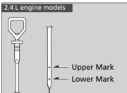
**4.** Remove the dipstick again, and check the level. It should be between the upper and lower marks. Add oil if necessary.
