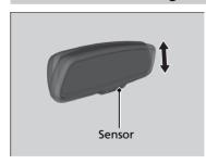
When driving after dark, the automatic dimming rearview mirror reduces the glare from headlights behind you. This feature is always active.
