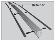
**4.** Remove the retainers from wiper blade and mount to a new rubber blade.
