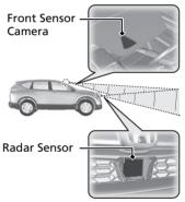
The radar sensor is inside the front grille.
