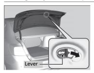
The trunk release lever allows you to open the trunk from inside for your safety.
