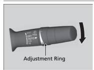
When you push the lever down to **AUTO**, the windshield wipers sweep once, and go into the automatic mode.
