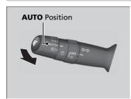
Disable the system when the vehicle is parked with the ignition switch in ON  $\overline{II}^{*1}$  and the light switch is in the **AUTO** position.
