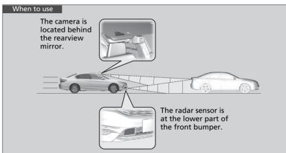
The system starts monitoring the roadway ahead when your vehicle speed is about 3 mph (5 km/h) and there is a vehicle in front of you.
