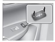
The ignition switch must be in ON [II]\*1 to use the seat heaters. The **HI** setting heats the seats faster than the **LO** setting.
