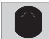
When the LKAS is suspended, the lane lines on the multi-information display change to contour lines, and the beeper sounds.
