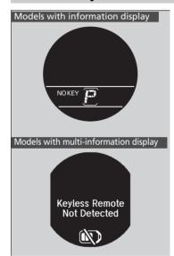
Warning buzzers may sound from inside and/ or outside the vehicle to remind you that the smart entry remote is out of the vehicle. If the buzzer continues even after the remote is put back inside, place it within the system's operational range.
