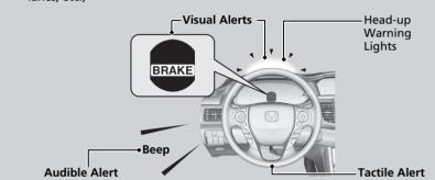
At system's earliest collision alert stage, you can change the distance (**Long/Normal/Short**) between vehicles at which alerts will come on through multi-information display setting options.
