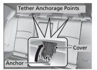
A tether anchorage point is provided behind each rear seating position. A child seat that is installed with a seat belt and comes with a tether can use the tether for additional security.
