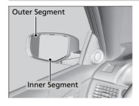
The driver side door mirror has outer and inner segments.
