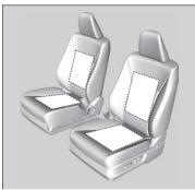
The ignition switch must be in ON  $\boxed{II}^{*1}$  to use the seat heaters. The HI setting heats the seats faster than the LO setting.
