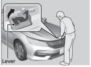
**3.** Push up the hood latch lever in the center of the hood to release the lock mechanism, and open the hood.
