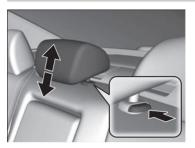
A passenger sitting in the center back seating position should adjust the height of their head restraint to an appropriate position before the vehicle begins moving.
