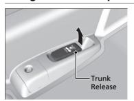
Pulling the trunk release to the lower left of the driver's seat unlocks and opens the trunk.
