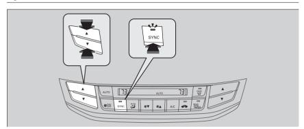
You can set the temperature synchronously for the driver side and the passenger side in synchronized mode.
