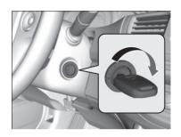
**3.** Turn the ignition switch to START **III** without depressing the accelerator pedal.
