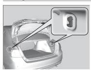
The cargo hooks in the trunk can be used to install a net for securing items.
