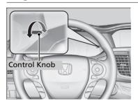
When the parking lights are turned on and the ignition switch is in ON [II]\*1, you can use the brightness control knob to adjust instrument panel brightness.
