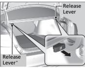
2. Pull the release lever in the trunk to release the lock
