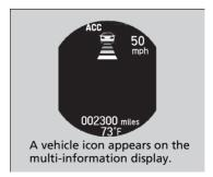
When a vehicle whose speed is slower than your set speed comes in or cuts in front of you and is detected by the radar, your vehicle starts to slow down.
