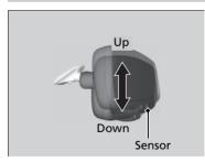
When driving after dark, the automatic dimming rearview mirror reduces the glare from headlights behind you, based in inputs from the mirror sensor. This feature is always active.
