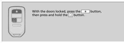
The engine runs for up to 10 minutes without you starting the vehicle.
