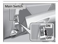
The trunk main switch disables the trunk release button on the remote transmitter and the trunk release button on the trunk lid to protect luggage in the trunk.
