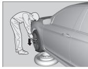
**6.** Loosen each wheel nut about one turn using the wheel nut wrench.
