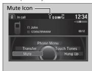
Press the **MENU** button to display the options. Rotate to select the mute option, then press .
