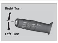
The turn signals can be used when the ignition switch is in ON  $\overline{II}$ <sup>\*1</sup>.
