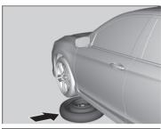
**5.** Place the compact spare tire (wheel side up) under the vehicle body, near the tire that needs to be replaced.
