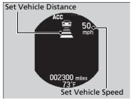
When ACC starts operating, the vehicle icon, distance bars and set speed appear on the multi-information display.
