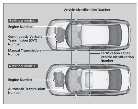
■ Vehicle Identification Number (VIN), Engine Number and Transmission Number
