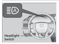
Turn the headlight switch in **AUTO** and pull the headlight lever to low beam.
