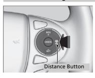
Press the (distance) button to change the ACC following-distance.
