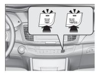
The rear defogger and heated door mirrors automatically switch off after 10-30 minutes depending on the outside temperature. However, if the outside temperature is 32°F (0°C) or below, they do not automatically switch off.
