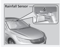
Do not put the wiper lever in **AUTO** when cleaning the windshield or driving through a car wash. If the wiper lever is in **AUTO**, and the power mode is in ON, the rainfall sensor may respond to your hand or car wash liquids, and the wipers may operate automatically.
