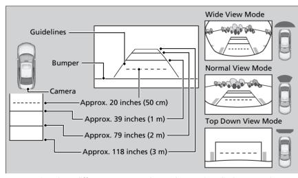
You can view three different camera angles on the rearview display. Press the selector knob or the interface dial to switch the angle.
