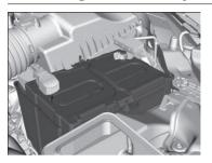
Check the battery terminals for corrosion monthly.
