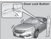
Press the door lock button on the front door.
