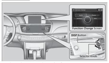
Press the **DISP** button to go to the **Function Change** screen. Rotate to select **Audio**, **Phone**, **Info** or **Settings** and press .
