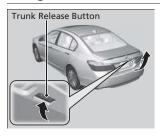
Push up the release button on the trunk lid after the doors are unlocked.
