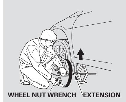
10. Use the extension and the wheel nut wrench as shown to raise the vehicle until the flat tire is off the ground.
