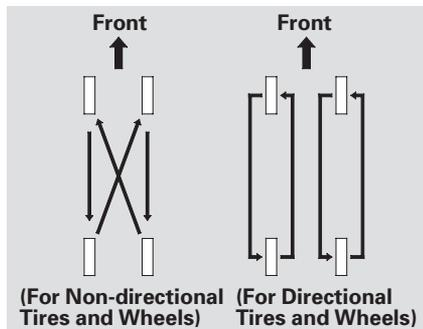
To help increase tire life and distribute wear more evenly, rotate the tires every 10,000 miles (16,000 km) on 4-cylinder models and 7,500 miles (12,000 km) on 6-cylinder models. Move the tires to the positions shown in the chart each time they are rotated. If you purchase directional tires, rotate only front-to-back.
