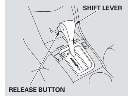
To shift from any position, press firmly on the brake pedal and press the release button on the side of the shift lever. You cannot shift out of Park when the ignition switch is in the LOCK (0) or ACCESSORY (I) position.
