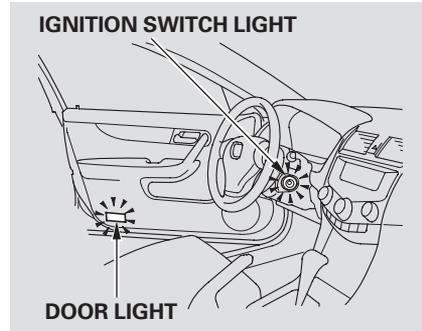
The courtesy light in each door comes on when the door is opened, and goes out when the door is closed.
