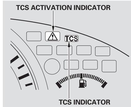
When starting out or driving on a loose or slippery road surface, you may notice that the vehicle does not respond to the accelerator in the same way it does at other times. This is a sign TCS is activating. You will see the TCS activation indicator flash.
