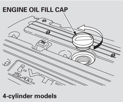
Unscrew and remove the engine oil fill cap on top of the valve cover. Pour in the oil slowly and carefully so you do not spill. Clean up any spills immediately. Spilled oil could damage components in the engine compartment.
