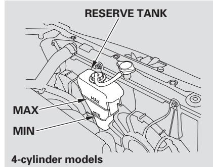
Look at the coolant level in the radiator reserve tank. Make sure it is between the MAX and MIN lines. If it is below the MIN line, see **Adding Engine Coolant** on page 217 for information on adding the proper coolant.
