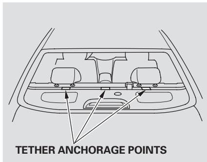
A child seat with a tether can be installed in any seating position in the back seat, using the anchorage points shown above.
