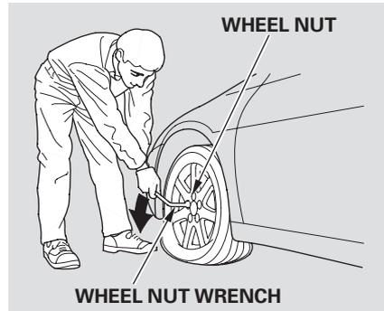
8. Loosen each wheel nut 1/2 turn with the wheel nut wrench.
