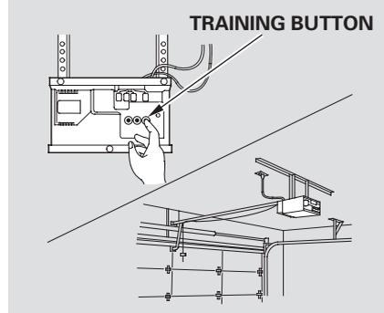
3. Press the training button on the garage door opener unit until the indicator next to the button comes on, then release it. The indicator may blink, or come on and stay on. You then have approximately 30 seconds to complete the following steps.
