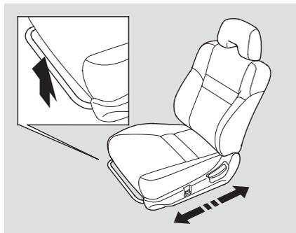
To adjust the seat forward and backward, pull up on the bar under the seat cushion's front edge. Move the seat to the desired position and release the bar. Try to move the seat to make sure it is locked in position.
