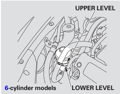
Pour the fluid slowly and carefully so you do not spill. Clean up any spill immediately; it could damage components in the engine compartment.
