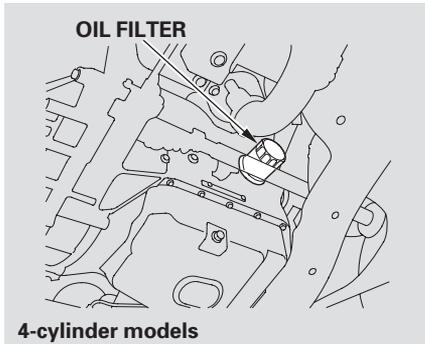
4. Install a new oil filter according to the instructions that come with it.
