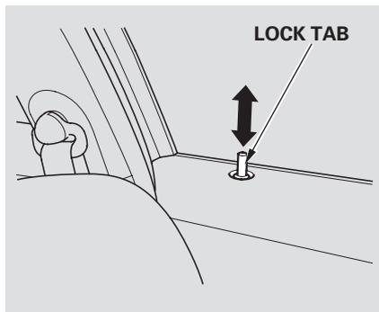
The lock tab on the passenger's door locks and unlocks only that door. Pulling up on the driver's door lock tab only unlocks the driver's door.
