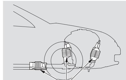
**THREE WAY CATALYTIC CONVERTERS**
