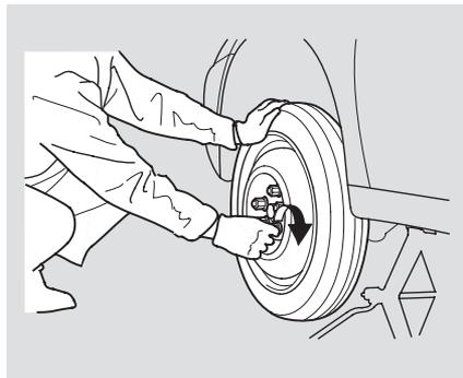
13. Put on the spare tire. Put the wheel nuts back on finger-tight, then tighten them in a crisscross pattern with the wheel nut wrench until the wheel is firmly against the hub. Do not try to tighten them fully.
