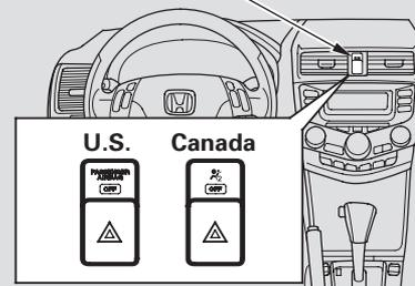
This indicator alerts you that the passenger's front airbag has been shut off because weight sensors detect an infant or small child may be in the front passenger's seat. It does **not mean** there is a problem with the airbag.
