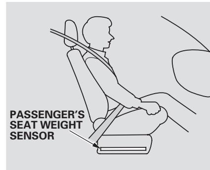
The passenger's advanced front airbag system has weight sensors under the seat. If the sensors detect an infant or small child may be in the seat, the system will automatically turn the passenger's front airbag off.
