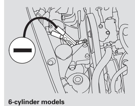
6. Start the vehicle. If the starter motor still operates slowly, check that the jumper cables have good metal-to-metal contact.
