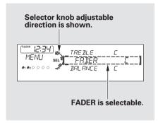
Press the MENU button to display the sound settings. Turn the selector knob to select an appropriate setting: bass, treble, fader, balance, SUBW\* (subwoofer) and SVC (speedsensitive volume compensation). Press the selector knob (ENTER) to enter the setting, then turn the selector knob to adjust the setting.
