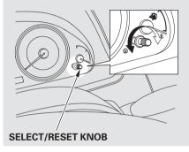
The select/reset knob on the instrument panel controls the brightness of the instrument panel lights. Turn the knob to adjust the brightness with the ignition switch in the ON (II) position and the parking lights on.
