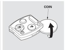
3. Inside the transmitter, separate the inner cover from the keypad by carefully prying on the edge with a coin.
