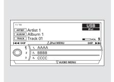
You can also change files with the interface dial. Press the AUDIO button to show the audio control display on the navigation screen. Push the selector to the right side to skip forward and to the left side to skip backward.
