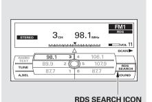
With the FM band selected, you can select the program type provided by the RDS. Press the AUDIO button to display the radio information on the screen. Push down the selector on the interface dial, then turn the knob to select RDS SEARCH icon. Press ENTER to set your selection. The principal RDS categories are shown as follows:
