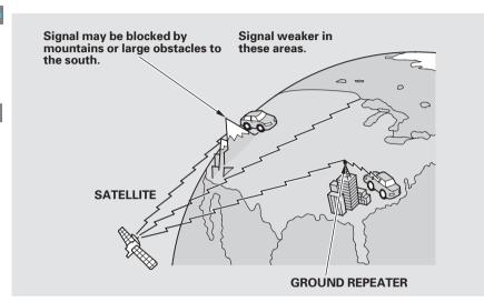
The XM satellites are in orbit over the equator; therefore, objects south of the vehicle may cause satellite reception interruptions. To help compensate for this, ground-based repeaters are placed in major metropolitan areas. Satellite signals are more likely to be blocked by tall buildings and mountains the farther north you travel from the equator. Depending on where you drive, you may experience reception problems. Interference can be caused by any of these conditions:
