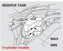
Look at the coolant level in the radiator reserve tank. Make sure it is between the MAX and MIN lines. If it is below the MIN line, see **Adding Engine Coolant** on page 348 for information on adding the proper coolant.
