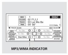
Using the interface selector, you can see the list of all the files and folders within a disc. While playing a MP3/WMA disc, press the AUDIO button. The currently playing folder and file information comes on the screen.
