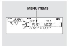
You can select any type of repeat, random and scan modes by using the MENU button and the selector knob. Push the MENU button to display the menu items, then turn the selector knob to select "PLAY MODE." Press the selector knob (ENTER) to set the selection.
