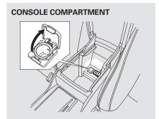
Each socket is intended to supply power for 12 volt DC accessories that are rated 120 watts or less (10 amps).
