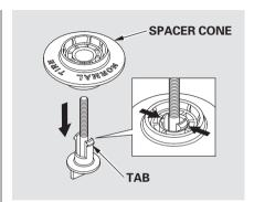
To remove the spacer cone, squeeze the tabs on the wing bolt to disengage it from the center of the spacer cone, then pull the bolt downward.
