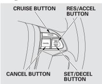
1. Push in the CRUISE button on the steering wheel. The CRUISE MAIN indicator on the instrument panel comes on.
