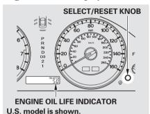
To see the current engine oil life. turn the ignition switch to the ON (II) position, then press and release the select/reset knob repeatedly until the engine oil life indicator appears (see page 66).
