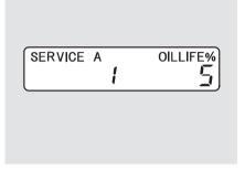
When the remaining engine oil life is 5 to 1 percent, you will see a "SERVICE" message along with the same maintenance item code(s). every time you turn the ignition switch to the ON (II) position.
