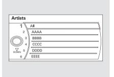
Push ENTER on the selector to display the items on that list, then turn the knob on the interface dial to select a desired list. Pushing the selector up or down moves a selection to the top or bottom of the screen items. Press ENTER to set your selection.
