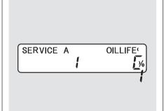
When the remaining engine oil life is 0 percent, the engine oil life indicator will blink. The display comes on every time you turn the ignition switch to the ON (II) position. The Maintenance Minder indicator ( so ) also comes on and remains on in the instrument panel. When you see this message, immediately have the indicated maintenance done by your dealer.
