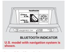
On models with navigation system A notification that there is an incoming call, or HFL is in use, will appear on the navigation screen when the audio system is on.
