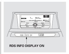
To switch the function between on and off, press and release the TITLE button. With the system on, you will see the "RDS INFO ON" message on the display. If the station you are listening to is an RDS station, the display shows the station name.
