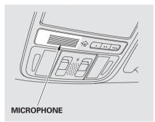
Air or wind noise from the dashboard and side vents, windows and moonroof may interfere with the microphone.
