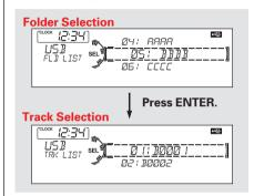
You can also select a folder or file from the list by using the selector knob. Push the selector knob (ENTER) to switch the display to the folder list, then turn the selector knob to select a folder. Press ENTER to change the display to the file list, then turn the same knob to select a file. Press ENTER to set your selection.
