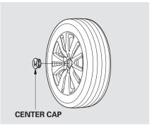
15.Remove the center cap (if equipped) before storing the flat tire in the trunk well.
