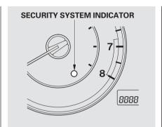
Once the security system sets, opening any door, the trunk, or hood without using the key or the remote transmitter, will cause the alarm to activate. It also activates if the ignition switch is turned to the ON (II) position, the audio unit is removed from the dashboard, or the wiring is cut.
