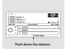
You can select any type of repeat and random mode on the audio menu. Press the AUDIO button to display the audio control screen, then push down the selector to display the audio menu. Turn the knob on the interface dial to select an audio mode: repeat, album random, and track random. Press ENTER to set your selection.
