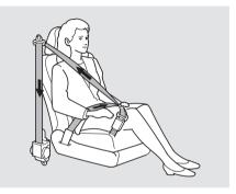
For added protection, the front seat belts are equipped with automatic seat belt tensioners. When activated, the tensioners immediately tighten the belts to help hold the driver and a front passenger in position. The tensioners can be activated during a collision in which the front airbags *do not deploy*. In this case, the airbags would not be needed, but the additional restraint could be helpful.
