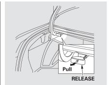
To release the seat-back from inside the trunk, pull the release under the trunk panel. Push the seat-back down from inside the trunk, or pull the seat-back down from inside the vehicle.
