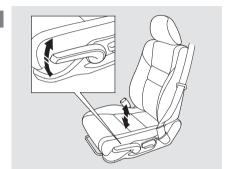
The height of your driver's seat is adjustable. To raise the seat, repeatedly pull up the lever on the outside of the seat cushion. To lower the seat, push the lever down repeatedly.
