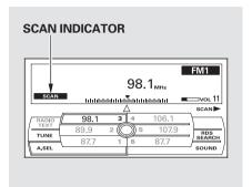
SCAN — The SCAN function samples all stations with strong signals on the selected band. To activate it, press the SCAN side of the SCAN/A.SEL bar, then release it.
