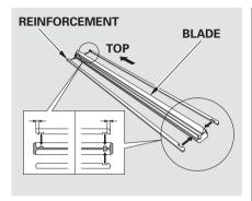
Make sure the three rubber tabs inside the blade fit to each notch of the reinforcement, as shown.
