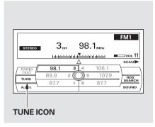
**TUNE** — Use the TUNE bar to tune the radio to a desired frequency. Press the right side of the bar to tune to a higher frequency, or the left side to tune to a lower frequency. To tune with the interface dial, push the selector down, and turn the knob to the TUNE icon. Then press ENTER on the selector, and turn the knob to the desired frequency. To exit the TUNE mode, press ENTER on the selector, then push the selector up.
