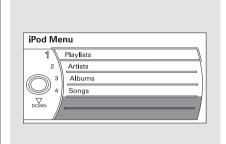
You can also select a file from any of the iPod menus: playlists, artists, albums and songs, by using the interface dial. Press the AUDIO button to display the audio control display on the navigation screen. Push up the interface selector to display the iPod menu. Turn the knob on the interface dial to select a desired list.
