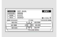
To listen to XM Radio, turn the ignition switch to the ACCESSORY (I) or ON (II) position, and press the (('>m')) button. The last channel you listened to will show in the audio screen and the center display. Adjust the volume by turning the power/volume knob.
