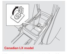
When you plug in a mini-jack cable between a compatible audio unit and the jack, you will see AUX in the display and the system automatically switches to AUX mode.
