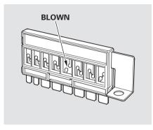
Also check the combined fuse box in the under-hood fuse box.
