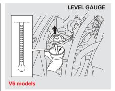
Fill the reservoir with a good-quality windshield washer fluid. This increases the cleaning capability and prevents freezing in cold weather.
