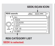
To activate RDS program search with the interface dial, push the AUDIO button to display the FM radio information on the screen. Push the selector down, and turn the knob to select the RDS SEARCH icon. Press ENTER on the selector. The screen shows you the RDS program category list.
