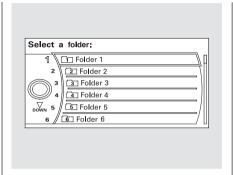
Push up the selector on the interface dial to switch the display to the folder list, then turn the knob on the interface dial to select a folder.
