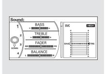
You can also adjust the sound by pushing the SOUND button repeatedly. Each mode is shown in the center display as it changes. Turn the power/volume knob to adjust the setting to your liking. When the level reaches the center, you will see "C" in the display. The system will return to the audio playing mode in the center display about 10 seconds after you stop adjusting a mode.
