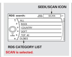
To activate RDS program scan with the interface dial, push the AUDIO button to display the FM radio information on the screen. Push the selector down, and turn the knob to select the RDS SEARCH icon. Press ENTER on the selector. The screen shows you the RDS category list.
