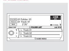
You can select any type of repeat, random and scan modes on the audio menu screen. Press the AUDIO button to show the audio control display on the navigation screen. Push down the selector on the interface dial to display the audio menu items.
