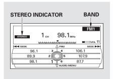
The ignition switch must be in the ACCESSORY (I) or the ON (II) position. Press the AUDIO button to view the audio control display. Turn the system on by pressing the power/volume knob or the FM/AM button. Adjust the volume by turning the power/volume knob.
