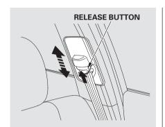
The front seats have adjustable seat belt anchors. To adjust the height of an anchor, press and hold the release button and slide the anchor up or down as needed (it has four positions). Never place the shoulder portion of a lap/shoulder belt under your arm or behind your back. This could cause very serious injuries in a crash.
