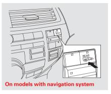
The defogger and antenna wires on the inside of the rear window can be accidentally damaged. When cleaning the glass, always wipe side to side.
