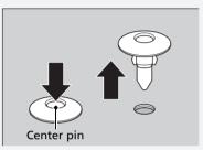
Push the center pin back to lock the clip. Then, insert the clip into the hole and press on the center pin until it is flat.
