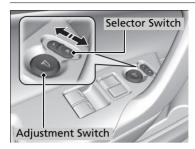
You can adjust the door mirrors when the ignition switch is in ON  $\boxed{II}^{*1}$ .
