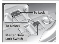
Press the master door lock switch in as shown to lock or unlock both doors.
