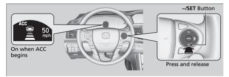
Take your foot off the pedal and press down the **–/SET** button when you reach the desired speed. The moment you release the button, the set speed is fixed, and ACC begins.
