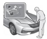
When finished, close the hood and make sure it is firmly locked in place.
