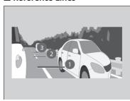
Three lines that appear on the screen can give an idea of how far the vehicles or objects on the screen are from your vehicle, respectively. If an object is near line 1 (in red), it indicates that it is close to your vehicle whereas an object near line 3 farther away.
