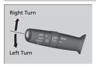
The turn signals can be used when the ignition switch is in ON II \*1.
