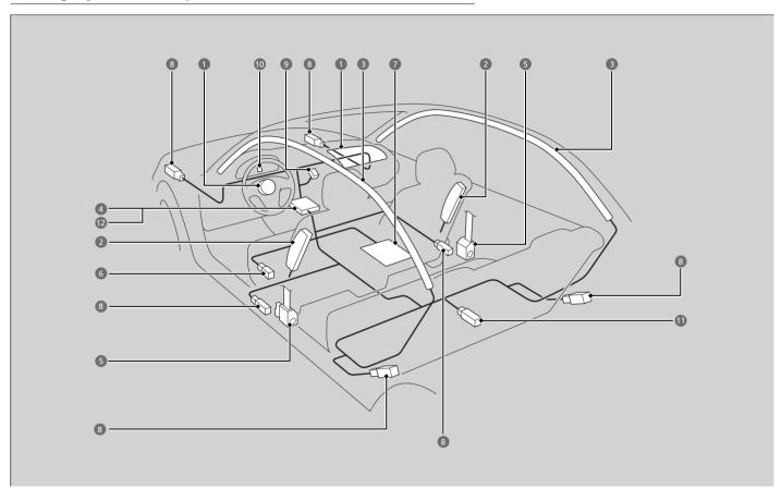
The front, front side, and side curtain airbags are deployed according to the direction and severity of impact. Both side curtain airbags are deployed in a rollover. The airbag system includes:
