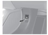
2 Locate the hood latch lever, pull the lever up, and lift up the hood.
