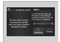
If your vehicle's airbags deploy or if the unit detects that the vehicle is severely impacted, your vehicle automatically will attempt to connect to the HondaLink operator. If connected, information about your vehicle, its location, and its condition will be sent to the operator; you also can speak to the operator when connected.
