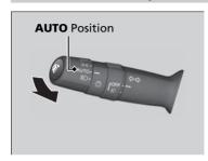
Disable the system when the vehicle is parked with the ignition switch in ON  $\boxed{II}^{*1}$  and the light switch is in the **AUTO** position.
