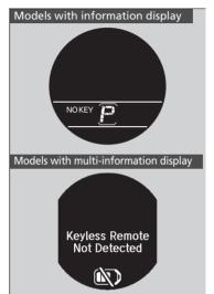
Warning buzzers may sound from inside and/ or outside the vehicle to remind you that the smart entry remote is out of the vehicle. If the buzzer continues even after the remote is put back inside, place it within the system's operational range.
