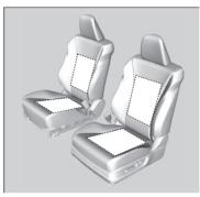
The ignition switch must be in ON [II]\*1 to use the seat heaters. The **HI** setting heats the seats faster than the **LO** setting.
