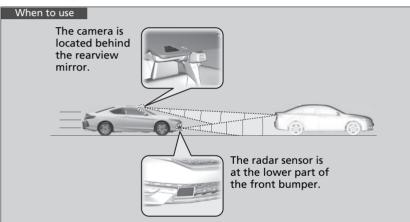
The system starts monitoring the roadway ahead when your vehicle speed is about 3 mph (5 km/h) and there is a vehicle in front of you.
