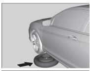
**5.** Place the compact spare tire (wheel side up) under the vehicle body, near the tire that needs to be replaced.
