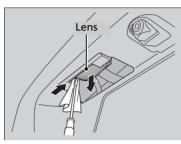
**1.** Remove the lens by carefully prying on its left edge with a small flat-tip screwdriver.
