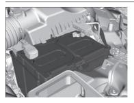
Check the battery terminals for corrosion monthly.
