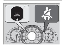
Your vehicle monitors front seat belt use. If the ignition switch is turned to ON  $\boxed{II}^{*1}$  before the driver's seat belt is fastened, the beeper will sound and the indicator will blink. If the driver does not fasten the belt before the beeper stops, the indicator will remain on.
