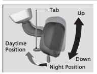
Flip the tab to switch the position.
