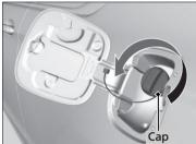
**4.** Remove the fuel fill cap slowly. If you hear a release of air, wait until this stops, then turn the knob slowly to open the fuel fill cap.
