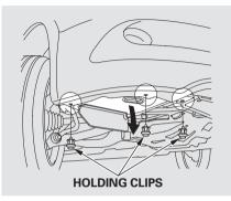
1. *Passenger's side* Remove the three holding clips with a flat-tip screwdriver.
