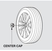
15.Remove the center cap (if equipped) before storing the flat tire in the trunk well.
