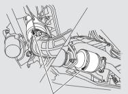
THREE WAY CATALYTIC CONVERTERS 4-cylinder models
