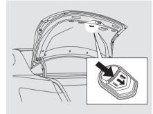
As a safety feature, your vehicle has a release lever on the trunk latch so the trunk can be opened from the inside.
