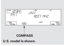
The compass may need to be manually calibrated after exposure to a strong magnetic field. If the compass seems to be continually showing the wrong direction and is not self-calibrating, or the compass display is blinking with the CAL indicator on, do the following.
