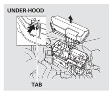
The under-hood fuse box is on the driver's side. To open it, push the tabs as shown.
