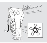
14. Tighten the wheel nuts securely in the same crisscross pattern. Have the wheel nut torque checked at the nearest automotive service facility. Tighten the wheel puts to:
