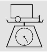
**Total Trailer Weight:** The maximum allowable weight of the trailer and everything in or on it must not exceed 1,000 lbs (450 kg). Towing a load that is too heavy can seriously affect your vehicle's handling and performance. It can also damage the engine and drivetrain.
