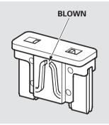
5. Look for a blown wire inside the fuse. If it is blown, replace it with one of the spare fuses of the same rating or lower.
