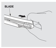
3. Remove the blade from its holder by grabbing the tabbed end of the blade. Pull firmly until the tabs come out of the holder. 4. Examine the new wiper blades. If they have no plastic or metal reinforcement along the back edge, remove the metal reinforcement strips from the old wiper blade, and install them in the slots along the edge of the new blade.
