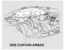
In a moderate to severe side impact, sensors will detect rapid acceleration and signal the control unit to instantly inflate the side curtain airbag.
