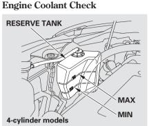
Look at the coolant level in the radiator reserve tank. Make sure it is between the MAX and MIN lines. If it is below the MIN line, see **Adding Engine Coolant** on page 356 for information on adding the proper coolant.
