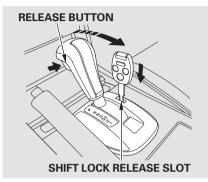
5. Push down on the key while you press the release button on the front of the shift lever and move the shift lever out of Park to neutral. 6. Remove the key from the shift lock release slot, then reinstall the cover. Make sure the notch on the cover is on the right side. Insert the key into the ignition switch, press the brake pedal, and restart the engine.
