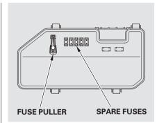
Your vehicle has spare fuses on the back of the under-hood fuse box cover.
