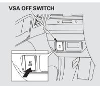
This switch is under the driver's side vent. To turn the VSA system on and off, press and hold it until you hear a beep.
