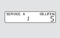
When the remaining engine oil life is 5 to 1 percent, you will see a "SERVICE" message along with the same maintenance item code(s), every time you turn the ignition switch to the ON (II) position. The maintenance item code or codes indicate the main and sub items required at the time of the oil change (see page 349).
