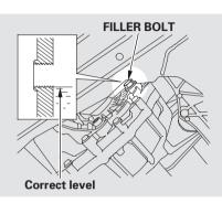
Remove the transmission filler bolt, and carefully feel inside the bolt hole with your finger.
