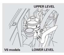
Pour the fluid slowly and carefully so you do not spill any. Clean up any spills immediately; it could damage components in the engine compartment. Always use Honda Power Steering Fluid. You may use another power steering fluid as an emergency replacement, but have the power steering system flushed and refilled with Honda PSF as soon as possible.
