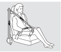
For added protection, the front seat belts are equipped with automatic seat belt tensioners. When activated, the tensioners immediately tighten the belts to help hold the driver and a front passenger in position. Driver and Passenger Safety
