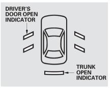
The appropriate indicator comes on if the trunk or any door is not closed tightly.
