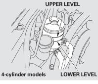
Check the level on the side of the reservoir when the engine is cold. The fluid should be between the UPPER LEVEL and LOWER LEVEL. If not, add power steering fluid to the UPPER LEVEL.
