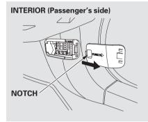
The passenger's side interior fuse box is on the lower passenger's side panel. To remove the fuse box lid, put your finger in the notch on the lid, and pull it upward slightly, then pull it toward you and take it out of its hinges.
