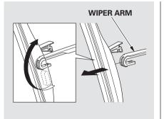
• Pivot the blade assembly toward the wiper arm until it releases from the wiper arm.
