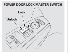
To lock all doors, push the front of the master door lock switch on either front door, pull the lock tab rearward on the driver's door, or use the key on the outside lock on the driver's door.
