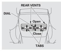
The airflow from the rear vents can be adjusted when the AUTO mode is selected or the fan mode is in the or position.
