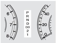
These indicators between the tachometer and speedometer show which position the shift lever is in.
