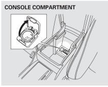
Each socket is intended to supply power for 12 volt DC accessories that are rated 120 watts or less (10 amps). None of the sockets will power an automotive type cigarette lighter element.
