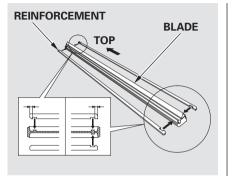
Make sure the three rubber tabs inside the blade fit to each notch of the reinforcement, as shown.
