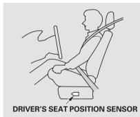
If there is a problem with the sensor, the SRS indicator will come on, and the airbag will inflate in the normal manner regardless of the driver's seating position.
