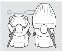
Your vehicle has a supplemental restraint system (SRS) with front airbags to help protect the heads and chests of the driver and a front seat passenger during a moderate to severe frontal collision (see page 23 for more information on how your front airbags work).
