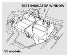
Check the terminals for corrosion (a white or yellowish powder). To remove it, cover the terminals with a solution of baking soda and water. It will bubble up and turn brown. When this stops, wash it off with plain water. Dry off the battery with a cloth or paper towel. Coat the terminals with grease to help prevent future corrosion. If additional battery maintenance is needed, see your dealer or a qualified mechanic.
