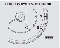
Once the security system is set, opening any door (without using the key or the remote transmitter), the hood, or the trunk will cause the alarm to activate. It will also activate if the audio unit is removed from the dashboard or the wiring is cut. With the system set, you can still open the trunk with the remote transmitter without triggering the alarm. The alarm will sound if the trunk lock is forced, or the trunk is opened with the trunk release lever or the emergency trunk opener.
