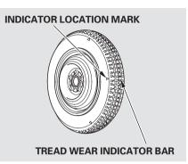
Replace the tire when you can see the tread wear indicator bars. The replacement should be the same size and design tire, mounted on the same wheel. The spare tire is not designed to be mounted on a regular wheel, and the spare wheel is not designed for mounting a regular tire. If you have a flat tire while driving, pull over safely. Drive slowly along the shoulder until you get to an area far away from traffic lanes.
