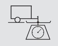
**Tongue Load:** The weight that the tongue of a fully-loaded trailer puts on the hitch should be approximately 10% of the total trailer weight. Too much tongue load reduces front-tire traction and steering control. Too little tongue load can make the trailer unstable and cause it to sway.
