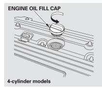
Unscrew and remove the engine oil fill cap on top of the valve cover. Pour in the oil slowly and carefully so you do not spill any. Clean up any spills immediately. Spilled oil could damage components in the engine compartment.
