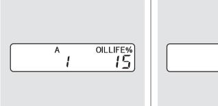
3. Press the select/reset knob for about 10 seconds. The engine oil life and the maintenance item code(s) will blink.  Press the select/reset knob for another 5 seconds. The maintenance item code(s) will disappear, and the engine oil life will reset to "100."
