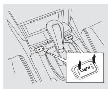
Push the right side of the switch, HI, to rapidly heat up the seat. After the seat reaches a comfortable temperature, select LO by pushing the left side of the switch. This will keep the seat warm. In the HI setting, the heater turns off when the seat gets warm, and turns back on after the seat's temperature drops.
