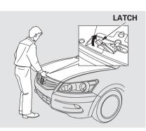
2. Reach in between the hood and the front grille with your fingers. The hood latch handle is above the "H" logo. Push this handle up until it releases the hood. Lift the hood. If the hood latch handle moves stiffly, or if you can open the hood without lifting the handle, the mechanism should be cleaned and lubricated.
