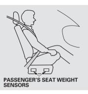
The passenger's advanced front airbag system has weight sensors under the seat. Although Honda does not encourage carrying an infant or small child in front, if the sensors detect the weight of an infant or small child (up to about 65 lbs or 29 kg), the system will automatically turn the passenger's front airbag off. Be aware that objects placed on the passenger's seat can also cause the airbag to be turned off.
