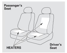
U.S. SE, EX-L and EX-L V6 Canadian EX-L and EX-L V6 Both front seats are equipped with seat heaters. Because of the sensors for the side airbag cutoff system, there is no heater in the passenger's seat-back. The ignition switch must be in the ON (II) position to use the heaters.
