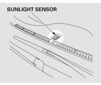
The climate control system has two sensors: a sunlight sensor on top of the dashboard, and a temperature sensor next to the steering column. Do not cover the sensors or spill any liquid on them.
