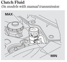
The fluid level should be between the MIN and MAX marks on the side of the reservoir. If it is not, add brake fluid to bring it up to that level. Use the same fluid specified for the brake system. A low fluid level can indicate a leak in the clutch system. Have this system inspected as soon as possible.
