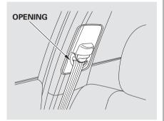
If your seat belts get dirty, use a soft brush with a mixture of mild soap and warm water to clean them. Do not use bleach, dye, or cleaning solvents. Let the belts air-dry before you use the vehicle. Dirt build-up around the openings of the seat belt anchors can cause the belts to retract slowly. Wipe the openings with a clean cloth dampened in mild soap and warm water or isopropyl alcohol. **Floor Mats**
