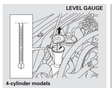
Check the level in the windshield washer reservoir at least monthly during normal use.
