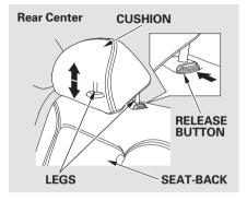
*Removing the Head Restraint* To remove a head restraint for cleaning or repair, pull it up as far as it will go. Push the release button, then pull the restraint out of the seatback.
