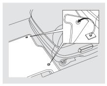
The driver's floor mat that came with your vehicle hooks over the floor mat anchors. This keeps the floor mat from sliding forward and possibly interfering with the pedals. Maintenance
