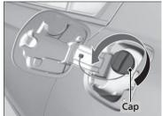
**4.** Remove the fuel fill cap slowly. If you hear a release of air, wait until this stops, then turn the knob slowly to open the fuel fill cap.
