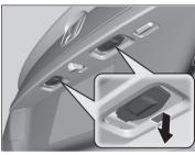
**1.** Remove the license plate light assembly by pushing the left edge of the lens toward the right and pulling the assembly out.
