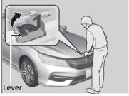
**3.** Push up the hood latch lever in the center of the hood to release the lock mechanism, and then open the hood.
