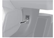
Locate the hood latch lever, pull the lever up, and lift up the hood.
