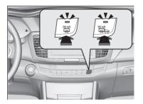
The rear defogger and heated door mirrors automatically switch off after 10-30 minutes depending on the outside temperature. However, if the outside temperature is 32°F (0°C) or below, they do not automatically switch off.
