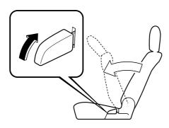
3. Raise the seatback to the most upright position. Make sure the seatback is securely latched by rocking the seatback.
