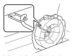
Secure the flat tire with the tire clamp and wing nut as shown below.
