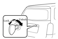
To unlock the liftgate with the key, insert the key and turn it clockwise.
