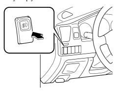
To turn on the fog lights, first turn on the headlight switch. Then press the fog light switch.
