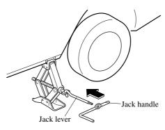
5. Turn the jack handle clockwise and raise the vehicle high enough so that the spare tire can be installed. Before removing the lug nuts, make sure your Mazda is firmly in position and that it cannot slip or move.
