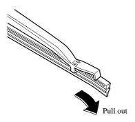
3. Remove the metal stiffeners from the blade rubber and install them in new blades.
