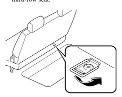
8. Install the flat tire with the tire securing bolt hooked in the anchor clip as shown below.
