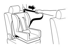
4. Push the child-restraint system firmly into the vehicle seat. Be sure the belt retracts as snugly as possible. Adjust the angle of the seat belt buckle so that the belt is not loose. Clicking from the retractor will be heard during retraction if the system is in the automatic locking mode. If the belt does not lock the seat down tight, repeat this step.
