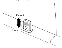
To lock a sliding door with the door-lock button from the outside, push down its door-lock button and close the door.
