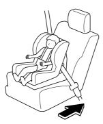
2. Secure the child-restraint system with the lap portion of the lap/shoulder belt. See the instructions on the child-restraint system for belt routing instructions.
