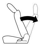
4. Expand the area between the seat bottom and the seatback slightly to verify the locations of the LATCH lower anchors.
