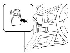
Press the switch again to turn the TCS back on. The TCS OFF indicator light will go out.
