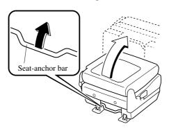
7. The seat is heavier than it looks, carefully pull up and detach the seat. Get assistance to lift it out of the vehicle.
