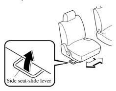
Make sure the lever returns to its original position and the seat is locked in place by attempting to push it from side to side.
