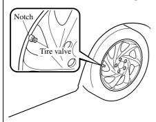
Damage could occur during installation if the wheel cover is not properly aligned.
