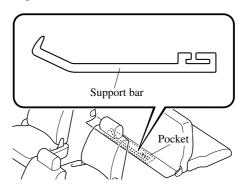
7. Set the hook on the support bar in the rear of the seatback.
