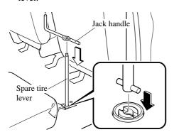
7. Slowly turn the handle counterclockwise until the spare tire reaches the ground and the cable becomes loose.
