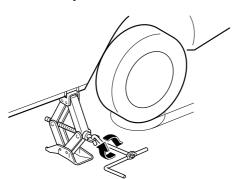
6. Remove the lug nuts by turning them counterclockwise; then remove the wheel.
