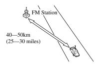
Signals from an FM transmitter are similar to beams of light because they do not bend around corners, but they do reflect.
