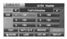
Each time the SAT1/2/3 on-screen button is pressed, the satellite selection changes in the order shown below.
